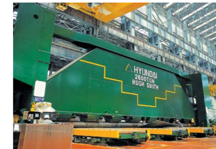
The world's largest CNC Roll Press makes it possible to roll side shell plates up to 21 m without welding seams.
