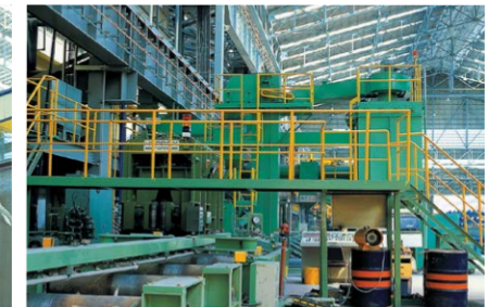
Profile and plate joints are mechanically blasted in the shop to remove rust, shop primer, and dampness to eliminate any possible welding defects.
