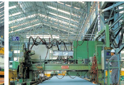
DNC (Direct Numerical Control) cutting machines to automate the character marking, cutting, feeding, and distribution of profiles and plates.
