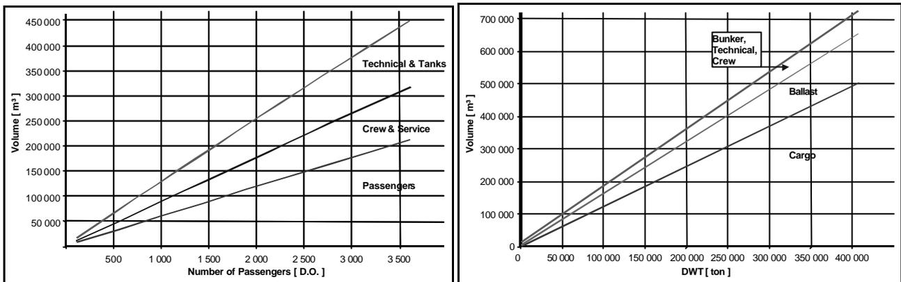
Figure 11: Total volume as a function of payload capacity for cruise ships and tankers
