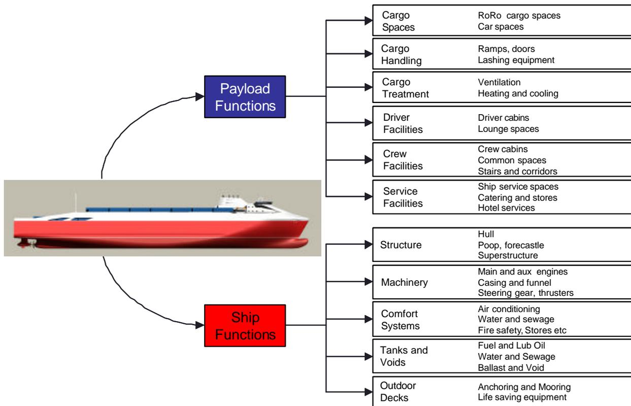
Figure 15: Payload and ship functions
