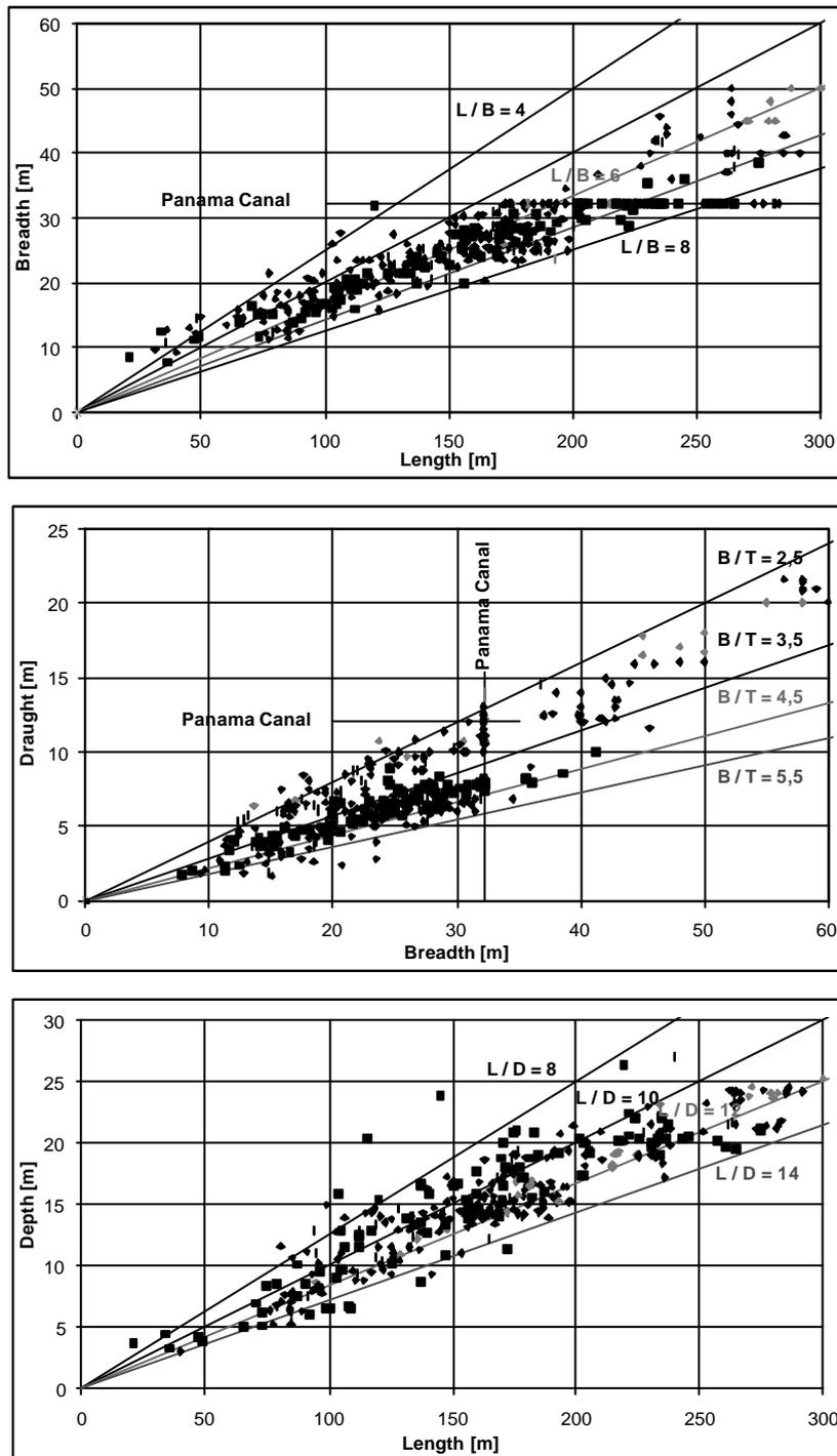
Figure 26: Main dimensions for ships with full displacement hull forms
