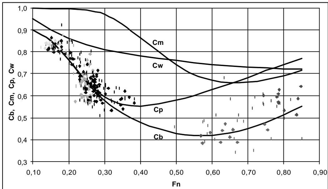
Figure 28: Hull coefficients
