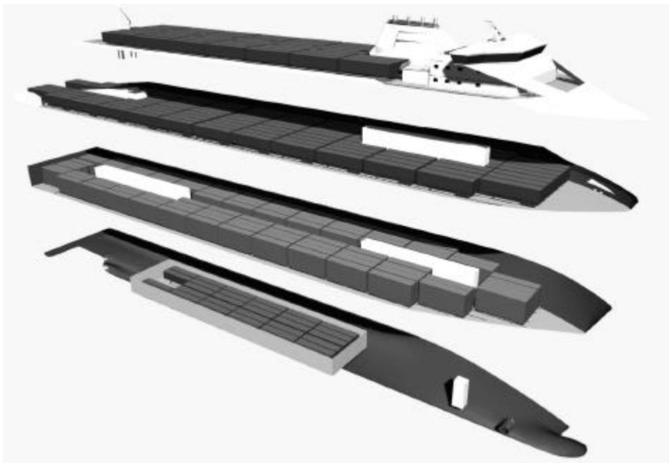
Figure 18: Enclosed and open cargo spaces
