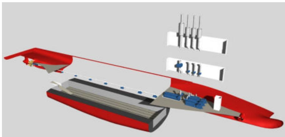
Figure 20: Machinery spaces, tanks and voids
