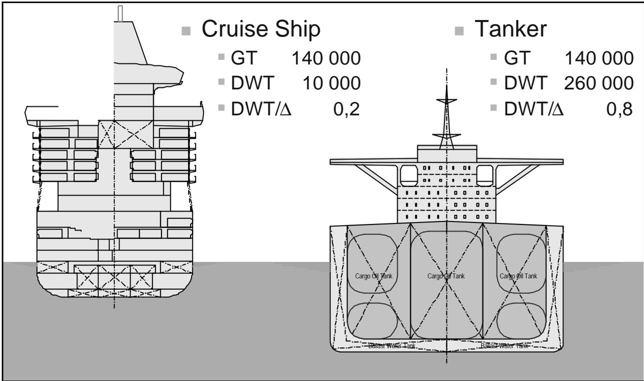
Figure 10: Cruise ships are capacity carriers, tankers are deadweight carriers
