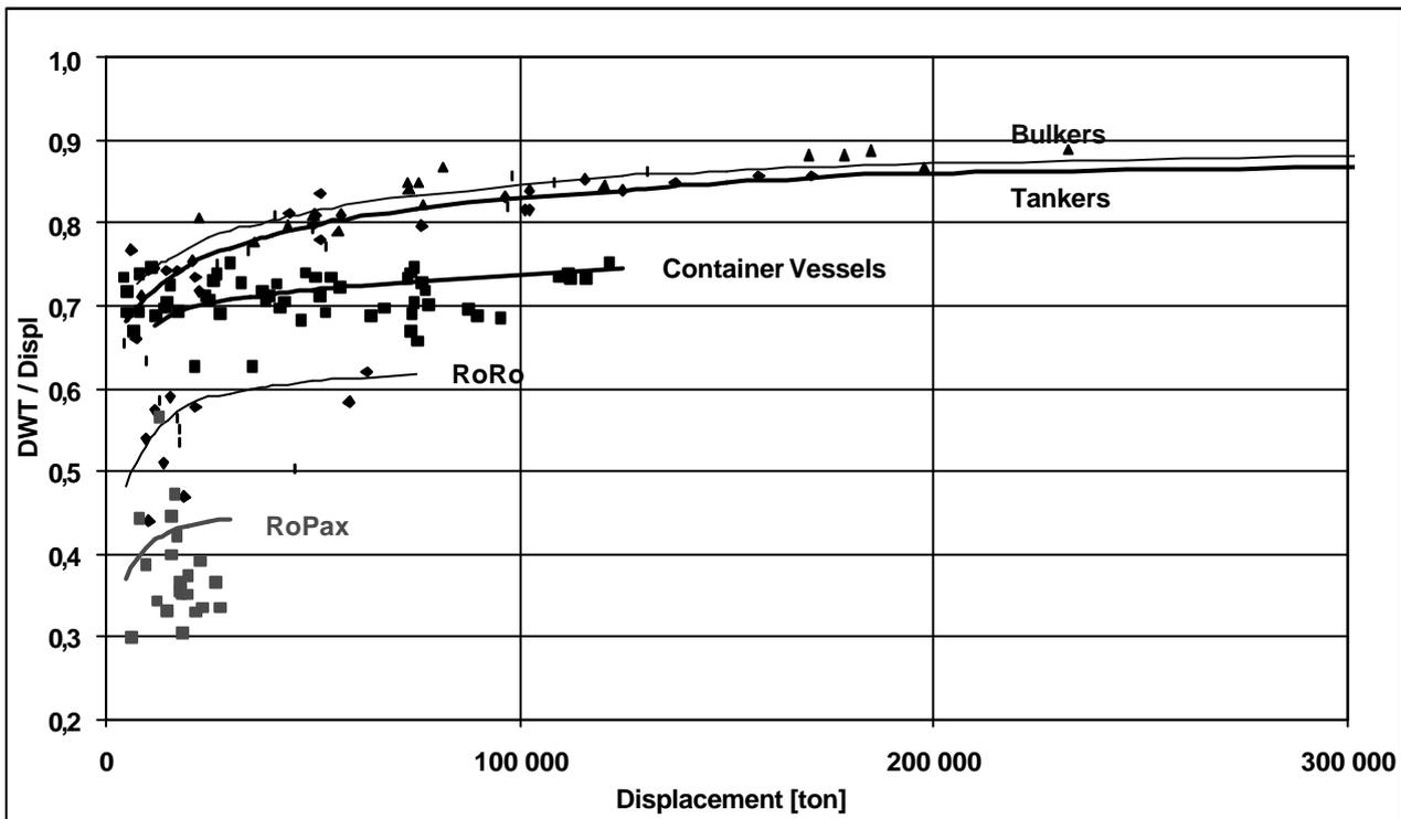
Figure 12: DWT / Displacement
