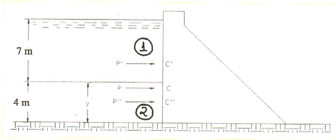
$$E_1 = \bar{P} \cdot A = \frac{(0 + 7000)}{2} \text{ kgf/m}^2 \times (7 \cdot 1) \text{ m} = \dots \text{ kgf/m de barragem}$$
