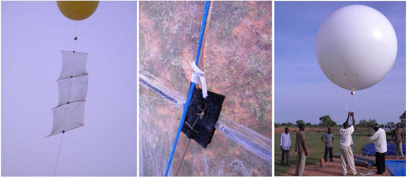
Extended Data Fig. 3 | Photograph showing a tethered sticky-panel setup and attachment. A sticky panel ( 3 \times 1 -m net) on a test helium balloon (of a lower volume and capacity), showing the attachment of the net covered with glue to the cord that tethers the balloon to the ground.
