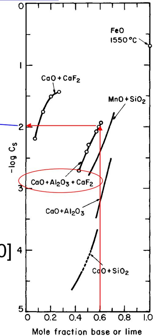
FIG. 22-18. Sulfide capacities of silicate, aluminate, and fluoride slags as a function of the mole fraction of the base at 1500°C; for CaO-Al<sub>2</sub>O<sub>3</sub>-CaF<sub>2</sub>, molar ratio Al<sub>2</sub>O<sub>3</sub>/CaF<sub>2</sub> = 1.3.<sup>[10]</sup>
