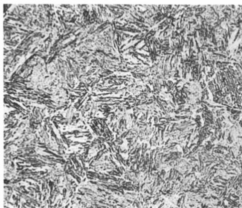
Fig. 1.7 10B35 steel austenitized 1 h at 850 °C (1560 °F) and quenched in agitated water. Tempered 1 h at 230 °C (450 °F). The structure is tempered martensite.
