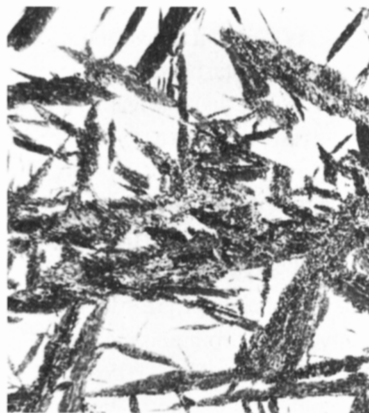
Fig. 1.6 1045 steel austenitized 10 min at 1205 °C (2200 °F), held 10 min at 340 °C (640 °F) for partial isothermal transformation, and cooled in air to room temperature. Lower bainite (dark) in a matrix of martensite (white). Picral etch. 500×
