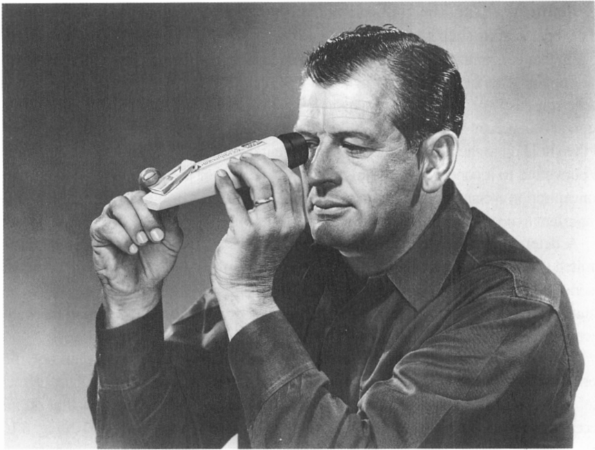
Fig. 6.15 Use of a hand-held refractometer. Courtesy of Leica Corporation
