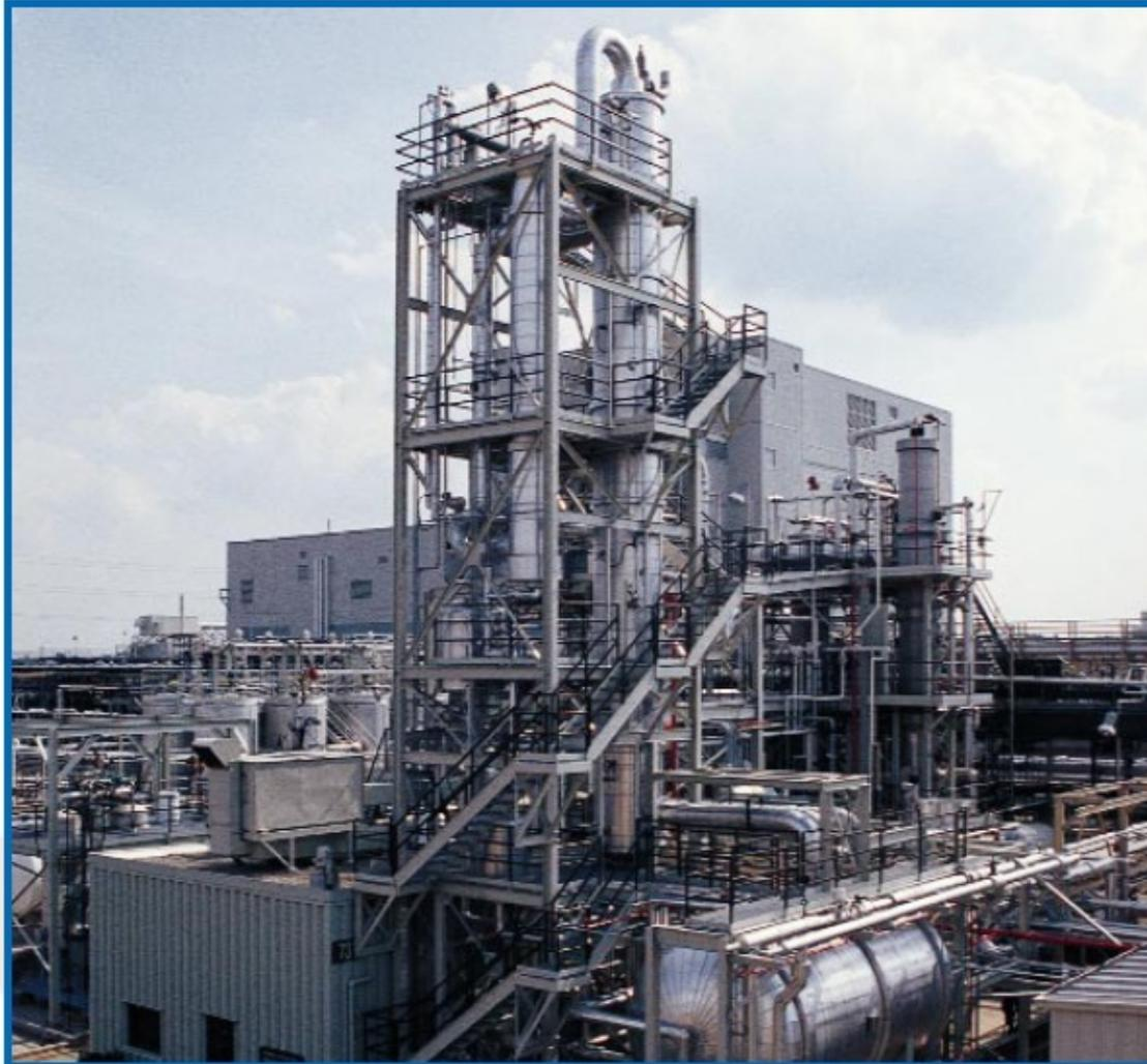
Figure 13. Batch distillation system.
