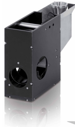
figure 31 DYNAMIC IMAGE ANALYSIS Particles fall in front of the zoom and basic cameras that capture digital images.
