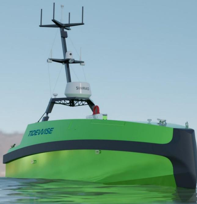
**USV Tupan** is an autonomous multi-purpose vessel designed and built in Brazil to operate in an offshore environment. Manufactured in aluminum and designed according to the UK MASS Rev3 guidelines.
