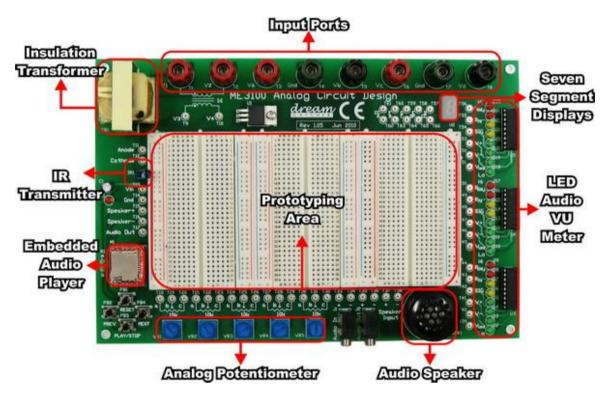
Figure A-1 – ME3100 Analog Circuit Design Kit
