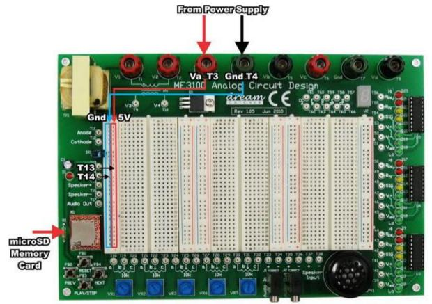
Figure 1 – Connections Between the Power Supply and the ME3100 Analog Circuit Design Kit
