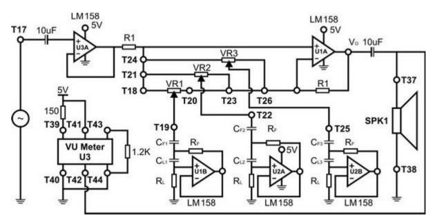
Figure 5 – Schematic Diagram of the 3-Band Gyrator-Based Equalizer with VU Meter
