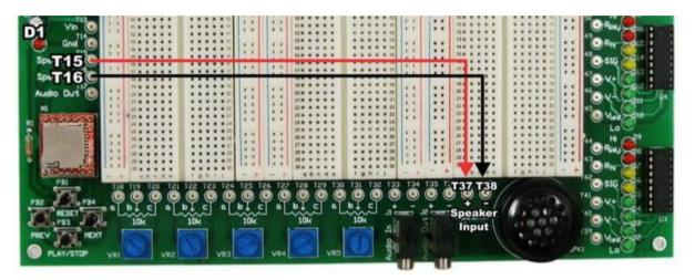
Figure 3 – Connections of T15 and T16 to the On-Board Speaker
