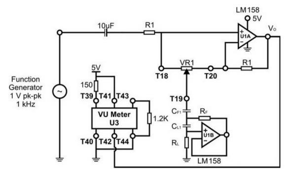
Figure 4 – Single Band Equalizer with VU Meter
