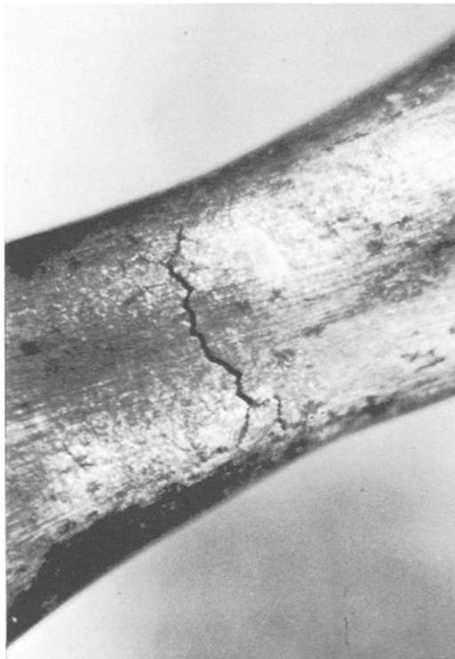
FIG. 2—Typical specimen surface at failure defined as a 10 to 20 percent decrease in steady state stress amplitude (X10).
