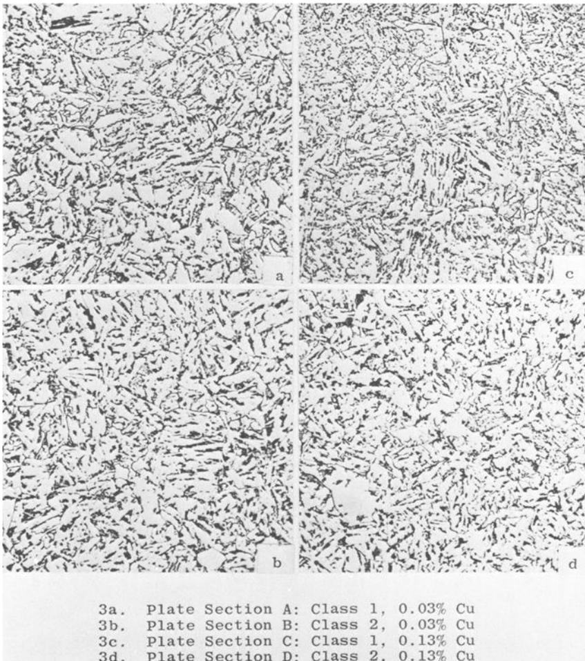
FIG. 3—Microstructures of plate sections A, B, C, and D (quarter thickness location). Structures appear very similar irrespective of the copper content variation. Tempered upper bainite ( $\times 500$ ; nital, picral etchant).
