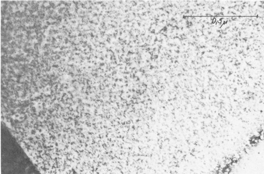
FIG. 12—Transmission electron micrographs of 16Cr-13Ni steel: top, unirradiated; bottom, irradiated at 50 C to  $0.8 \times 10^{22}$  n/cm<sup>2</sup>.
