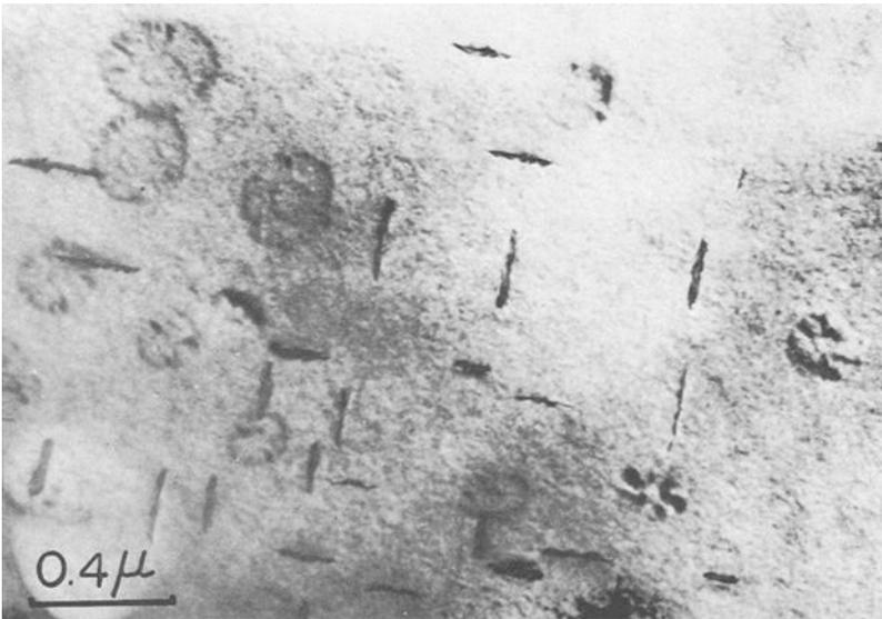
FIG. 5—*Stable precipitates which are formed after irradiation.*
