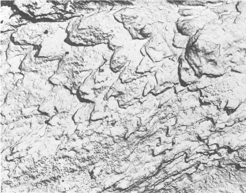
FIG. 11—Fracture surface of unirradiated Type 304 stainless steel tested at 750 C. Total elongation 35 percent ( $\times 7500$ ).
