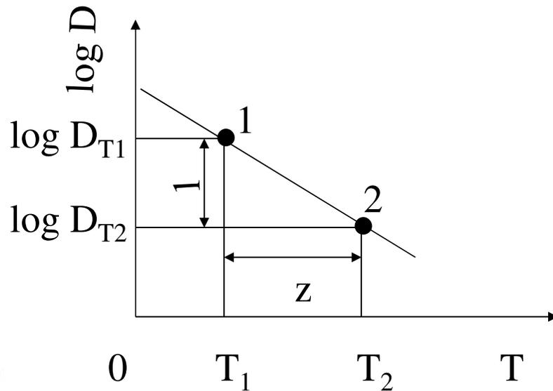
$$\log D_{T2} = \log D_{T1} - (1/z) (T_2 - T_1)$$
