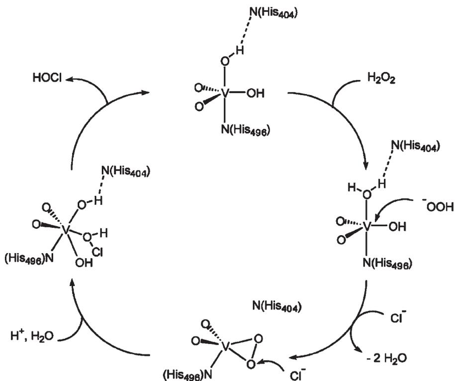
**Figure 17.14** Proposed mechanism for the vanadium chloroperoxidase oxidation of chloride by hydrogen peroxide. (From Ligtenberg et al., 2003. Copyright 2003, with permission from Elsevier.)
