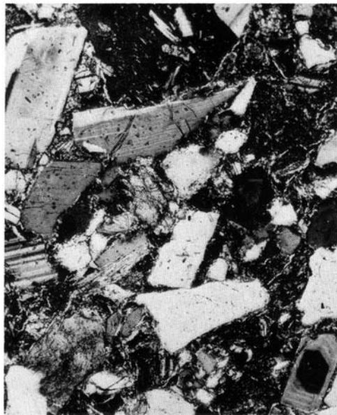
FIG. 2.—Feldspathic lithic (volcanic) wacke, Eocene Tyee Formation, east of Reedsport, Oregon. Both compositionally and texturally very immature (quartz 32%, feldspar 30%, volcanic rocks 13%, ferromagnesian minerals 12%, matrix 13%; standard deviation 1.45, average roundness 0.22). Crossed nicols, X63.
