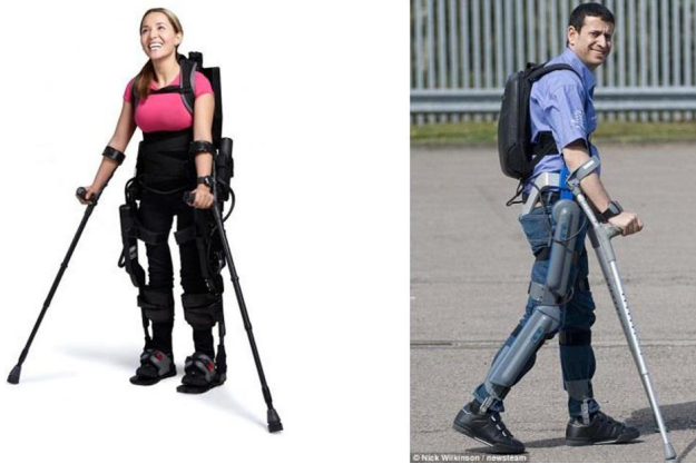
FIGURE 9.2.1 Robots allow spinal cord injured people to walk over ground, Ekso Bionics and ReWalk, courtesy, www.eksobionics.com and www.rewalk.com .
