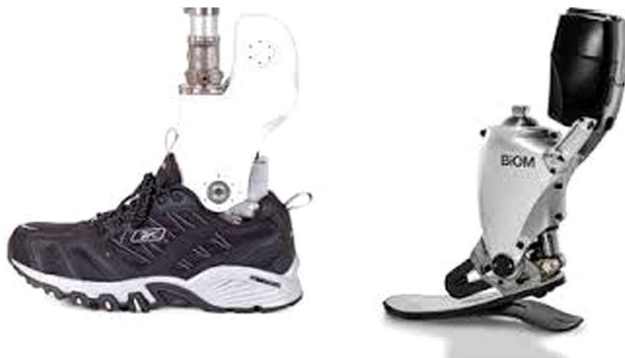
FIGURE 9.2.5 The Odyssey ankle is shown on the left and the Bionix ankle is shown on the right, courtesy of www.springactive.com and www.bionix.com .
