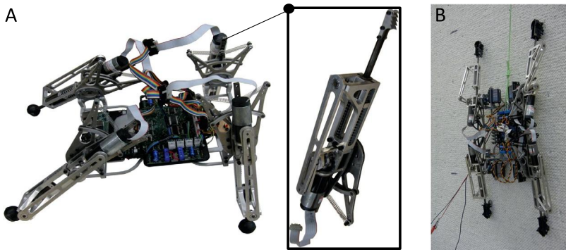
FIGURE 7.2.5 SCARAB, a quadrupedal running and climbing platform. (A) Running mode, (B) close up of the leg design, and (C) in climbing mode.
