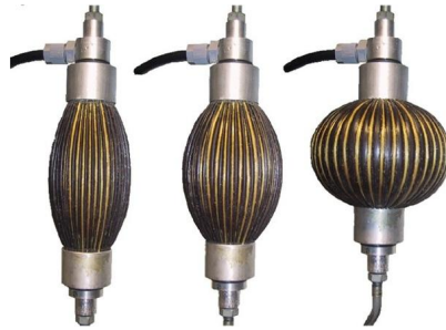
FIGURE 8.3.6 Pleated pneumatic artificial muscle (PPAM) developed by Vanderborght et al. in Free University of Brussels.
