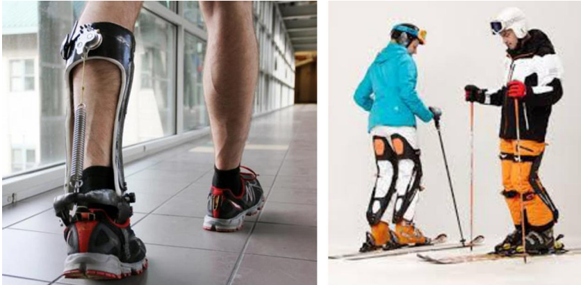
FIGURE 9.2.7 A passive ankle foot orthosis makes it easier to walk, reducing metabolic cost (Collins et al., 2015). The figure on the right shows an exoskeleton that reduces the load at the knees when skiing, courtesy of www.againer-ski.com .
