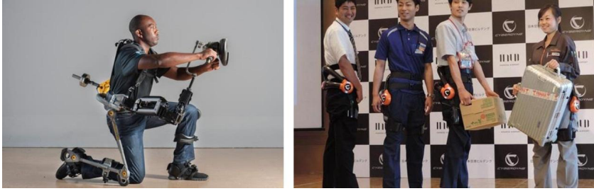
FIGURE 9.2.6 The Lockheed Martin Fortis device is shown on the left. It is a passive exoskeleton that transfers the load of the grinder to the ground, courtesy of http://www.lockheedmartin.com/us/products/exoskeleton/FORTIS.html . A hip exoskeleton makes it easier to carry luggage, courtesy of http://www.cyberdyne.jp/english/ .
