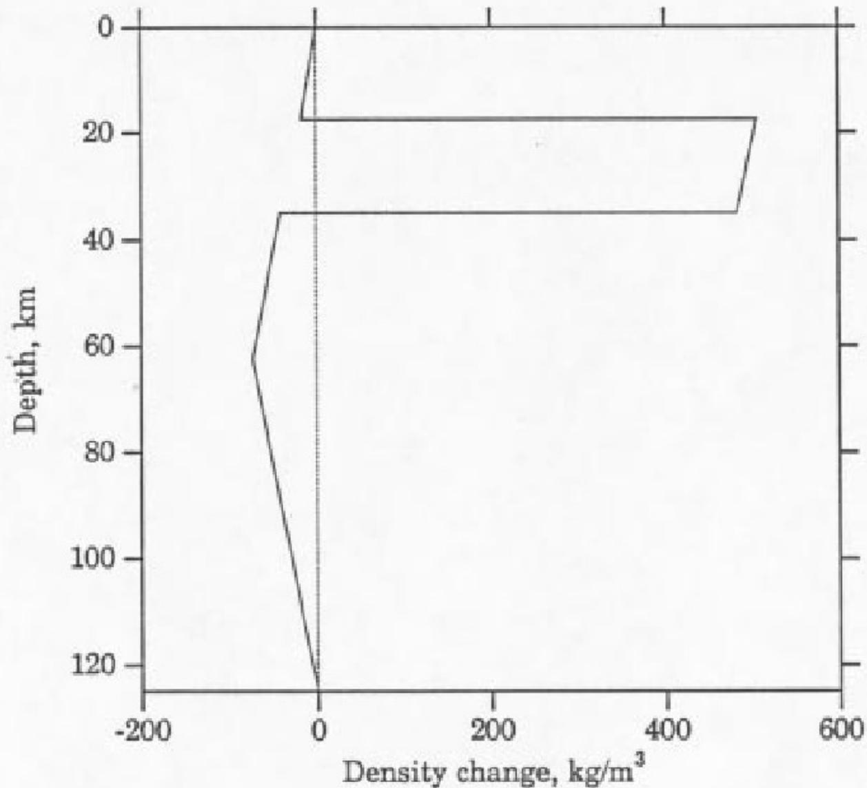
Figure 4.1 Density changes occur when lithosphere is stretched by  $\beta = 2$ . Original thickness of crust and lithosphere is 35 km and 125 km, respectively. Shallow zone of increased density is due to mantle lithosphere replacing crust. Zones of decreased density are due to heating of the crust and mantle lithosphere, and replacement of mantle lithosphere by asthenosphere.
