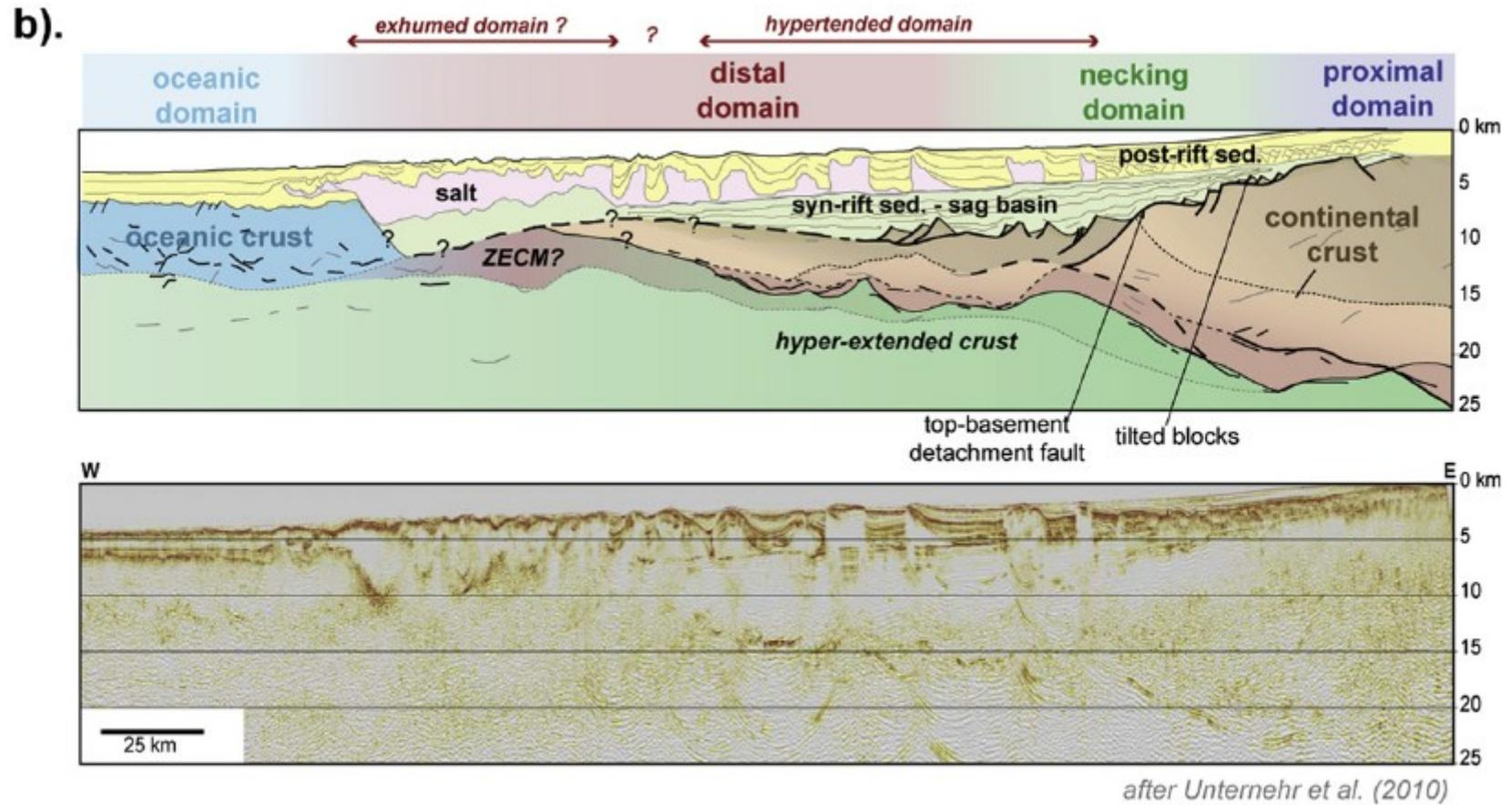
**Figure 9.** a: Bathymetric map of the Angola–Gabon margin with location of the presented section. b: Seismic reflection profile (courtesy of ion-GXT) and interpretation illustrating the main structural characteristics of the Angola–Gabon margin (segment 3) (after Unternehr et al., 2010).
