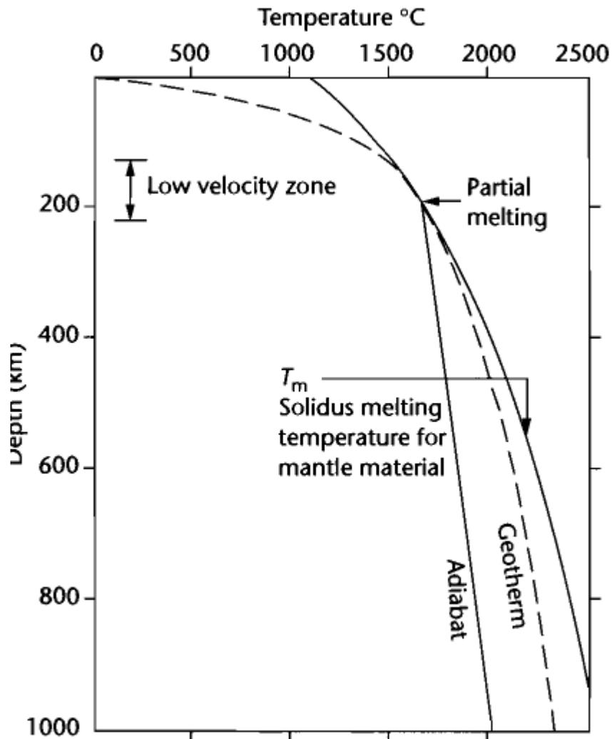
**Fig. 1.4** Variation of temperature with depth, or geotherm, and the solidus temperature for mantle material (peridotite). Where the solidus curve ( $T_m$ ) and the geotherm become tangential, partial melting in the mantle is likely to take place, resulting in a zone of low seismic wave velocities (low velocity zone).
