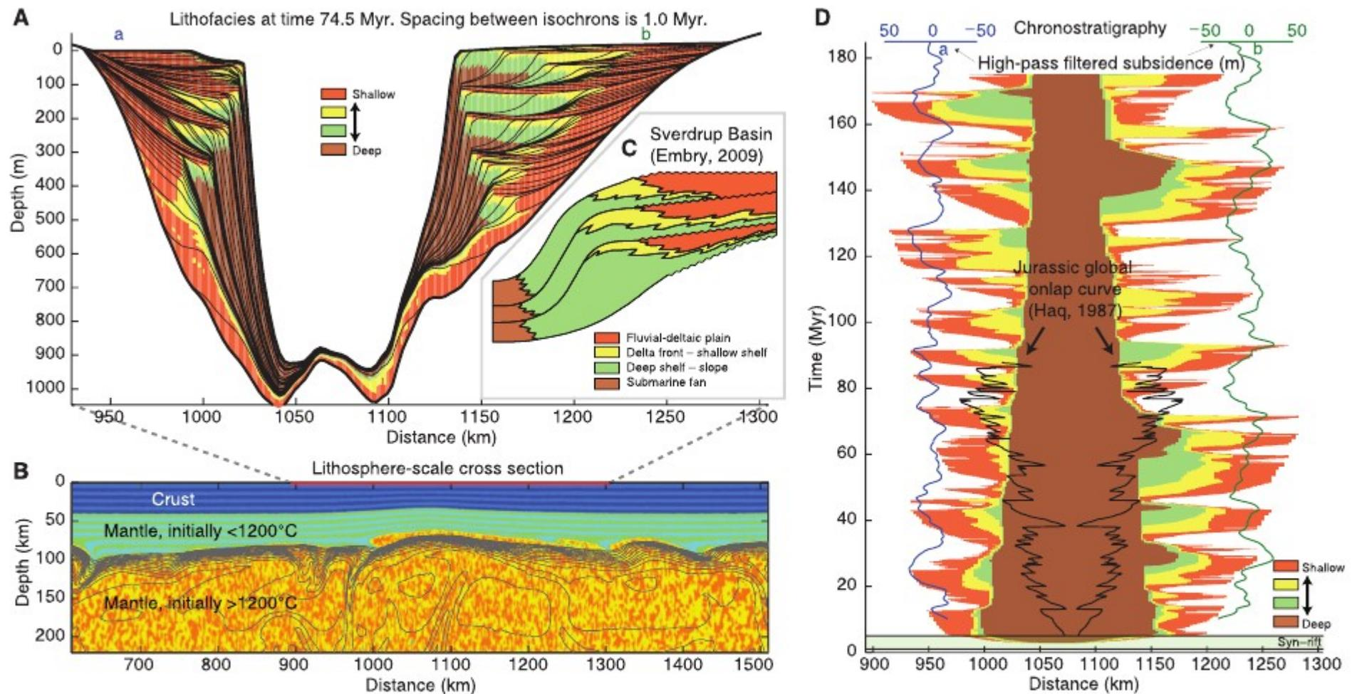
**Fig. 3.** Rift model with small-scale convection and constant sediment input and eustatic sea level. **(A)** Lithofacies (indicated by paleo water depth). Cyclic deposition is evident from unconformities and lateral migration of lithofacies; subsidence curves for locations a and b appear in **(D)**. **(B)** Lithospheric cross-section showing gently thinned crust and mantle lithosphere and isotherms from 1200° to 1440°C (solid lines). **(C)** Cross section of the Sverdrup Basin,
