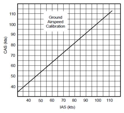
Figure 8 Ground Airspeed Calibration
