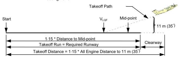
Figure 23–4 TAKEOFF RUN – All Engines Operating
