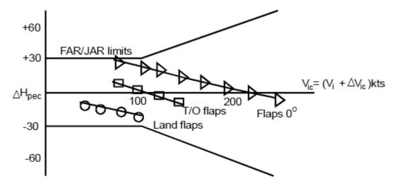
Figure 3 Typical Position Error Correction Data for an Aircraft
