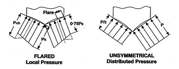
FIGURE 3. Transverse pressure distribution.
