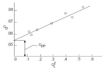
Figure 1 COEFFICIENT OF DRAG VERSUS COEFFICIENT OF LIFT
