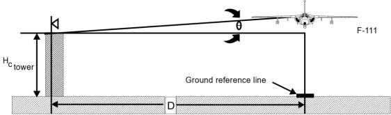
Figure 5 Tower Fly-By Method
