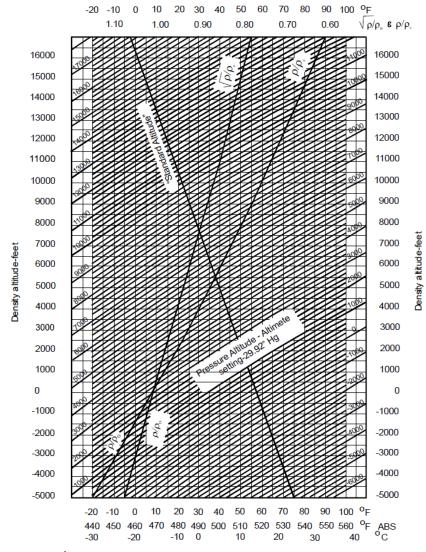
Figure 4 – DENSITY/PRESSURE ALTITUDE CONVERSION
