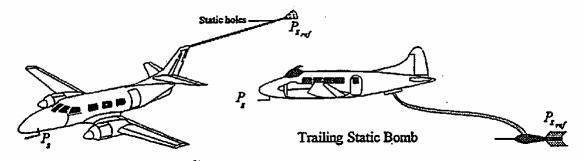
Figure 2 Sketches of Trailing Static Bomb and the Trailing Static Cone (not to scale)
