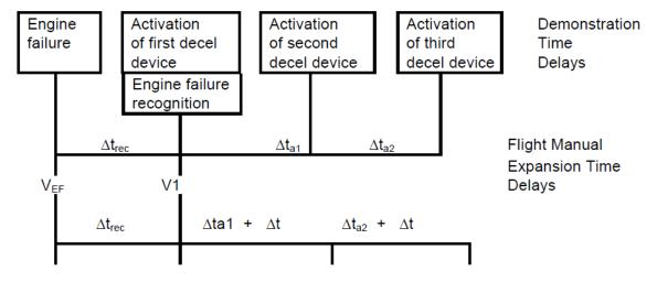
Figure 21-1 ACCELERATE-STOP TIME DELAYS
