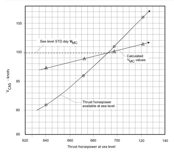
Figure 1 - THRUST HORSEPOWER AT SEA LEVEL
