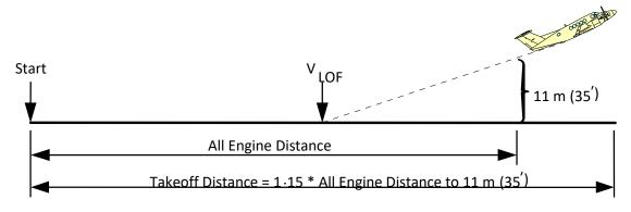
Figure 23–2 TAKEOFF DISTANCE – All Engines Operating
