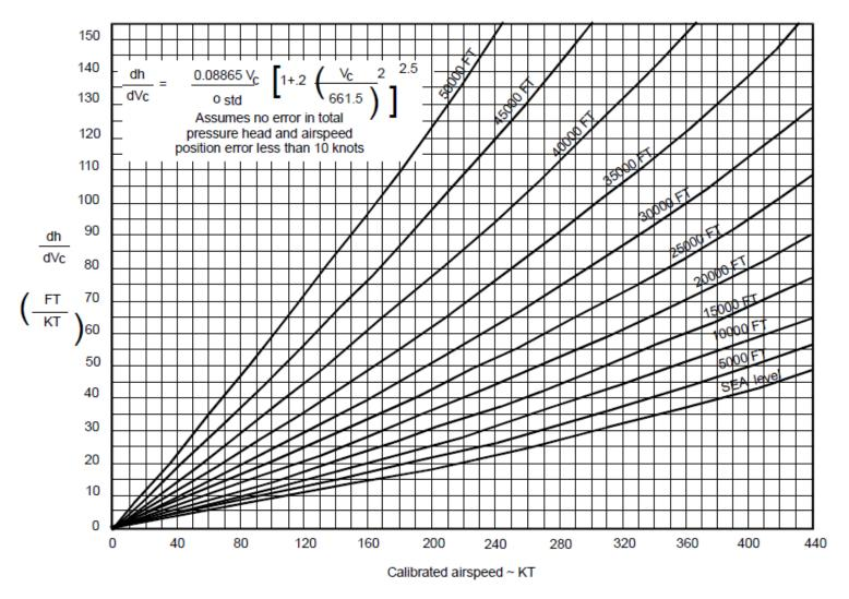
FIGURE 6 - ALTIMETER ERROR VS. CAS
