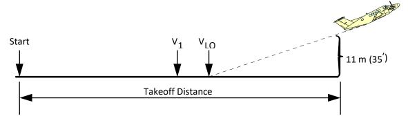
Figure 23–1 TAKEOFF DISTANCE Critical Engine Failure Recognised at V<sub>1</sub>
