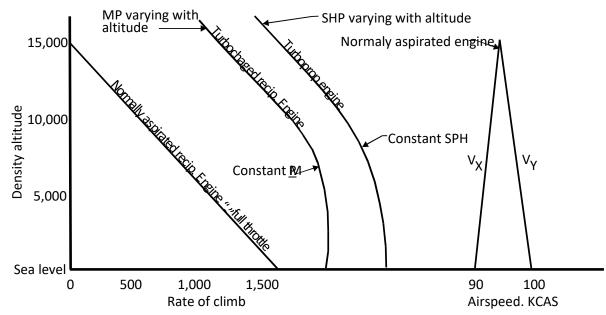
Figure 25-3 RATE OF CLIMB AND SPEEDS
