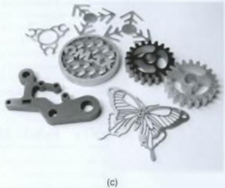
FIGURE 27.18 (a) Schematic illustration of the water-jet machining process. (b) A computer-controlled water-jet cutting machine. (c) Examples of various nonmetallic parts produced by the water-jet cutting process. Source: Courtesy of OMAX Corporation.
