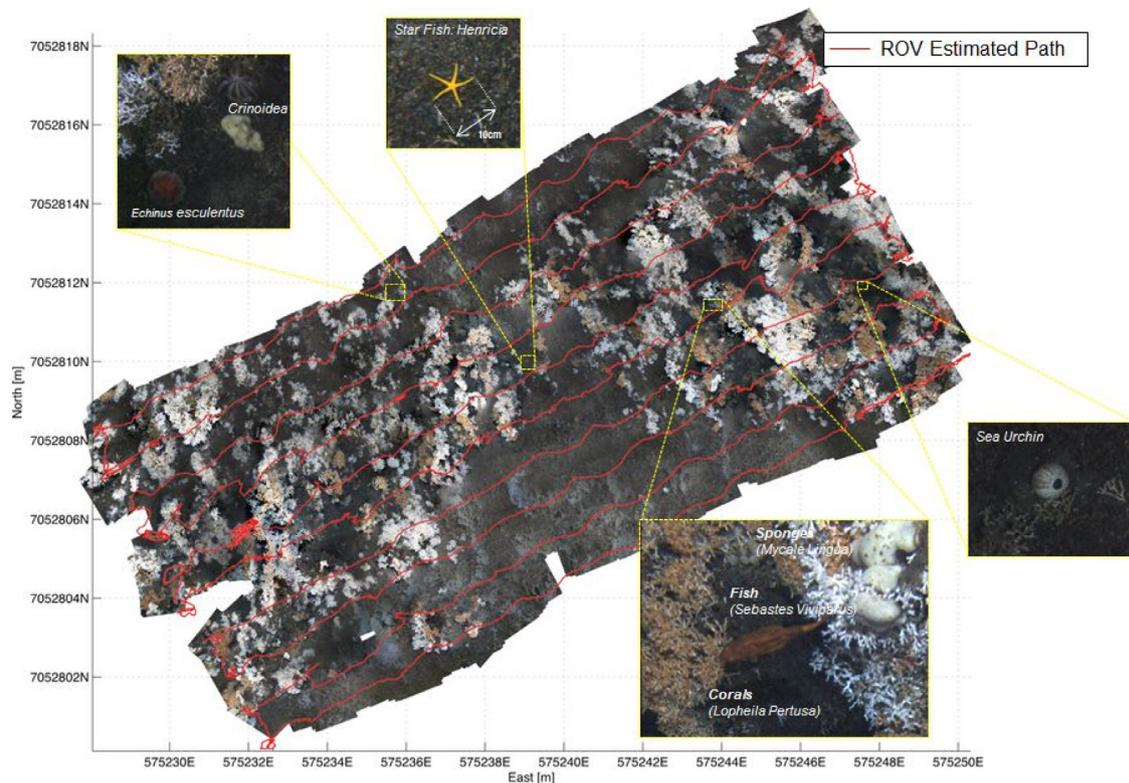
Fig. 9. Photomosaic from Taura coral reef captured using ROV minerva with path following capability.
