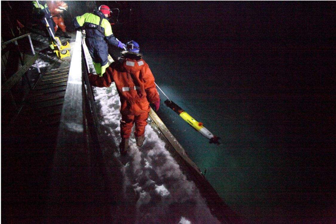
Fig. 6. Recovery of the REMUS AUV after a successful mission measuring vertical zooplankton distribution.
