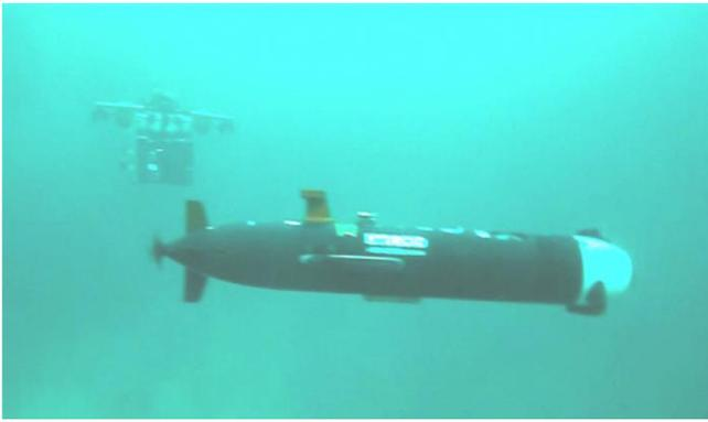
Fig. 3. AUV REMUS and ROV minerva together.
