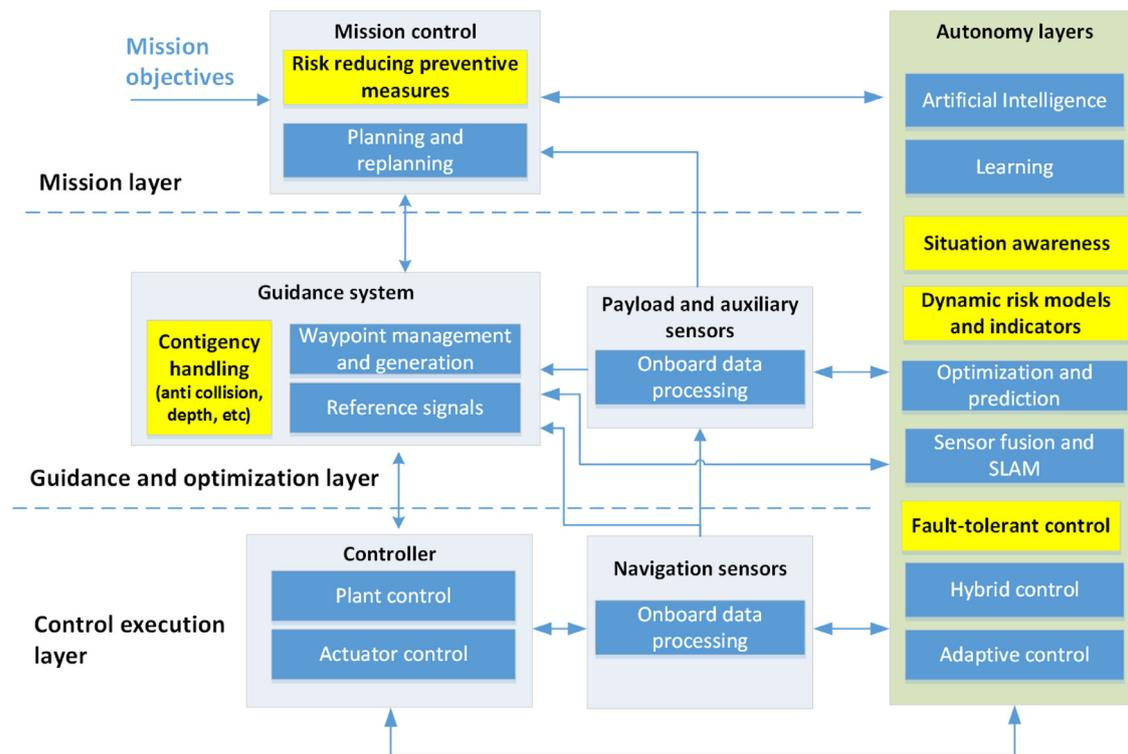
Fig. 8. Control architecture for unmanned underwater vehicles.
