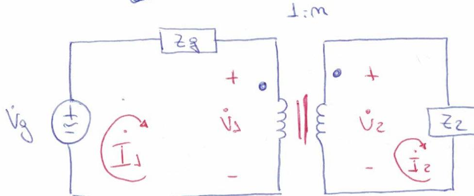
$$\frac{\dot{V}_2}{\dot{V}_1} = m \quad \frac{\dot{I}_2}{\dot{I}_1} = \frac{1}{m} \quad \frac{Z_2}{Z_1} = m^2$$
