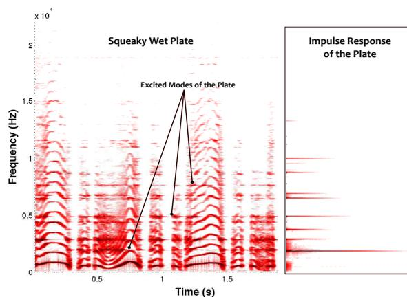
Figure 5: *Squeaky Wet Plate and its Impulse Response*
