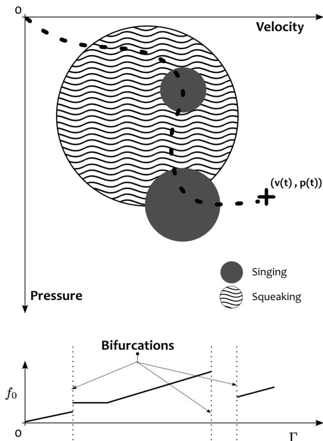
Figure 7: An Example of Control Strategy by Defining the Vibrating Behavior According to Velocity / Pressure Areas and the Mapping Function Between the Descriptors  $\gamma$  and the Fundamental Frequency  $f_0$
