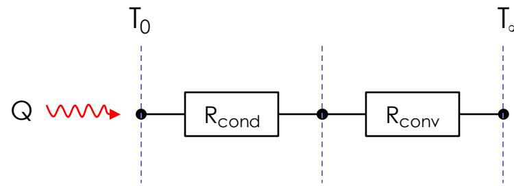
$$Q = \frac{T_{\text{sup}} - T_{\infty}}{\frac{L}{kA_{\text{cond}}} + \frac{1}{hA_{\text{conv}}}}$$
