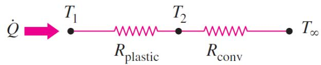
$$R_{\text{total}} = R_{\text{plastic}} + R_{\text{conv}} = 0.76 + 0.18 = 0.94 \text{ }^{\circ}\text{C/W}$$
