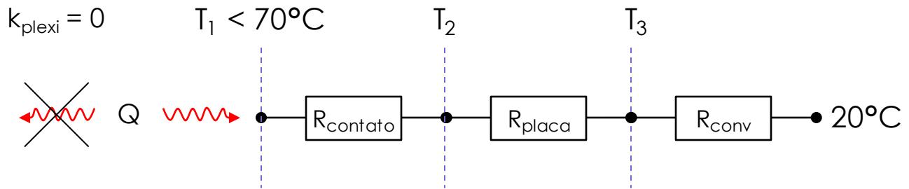
$$R_{total} = R_{contato} + R_{placa} + R_{conv} = 4.0326^\circ\text{C/W}$$
