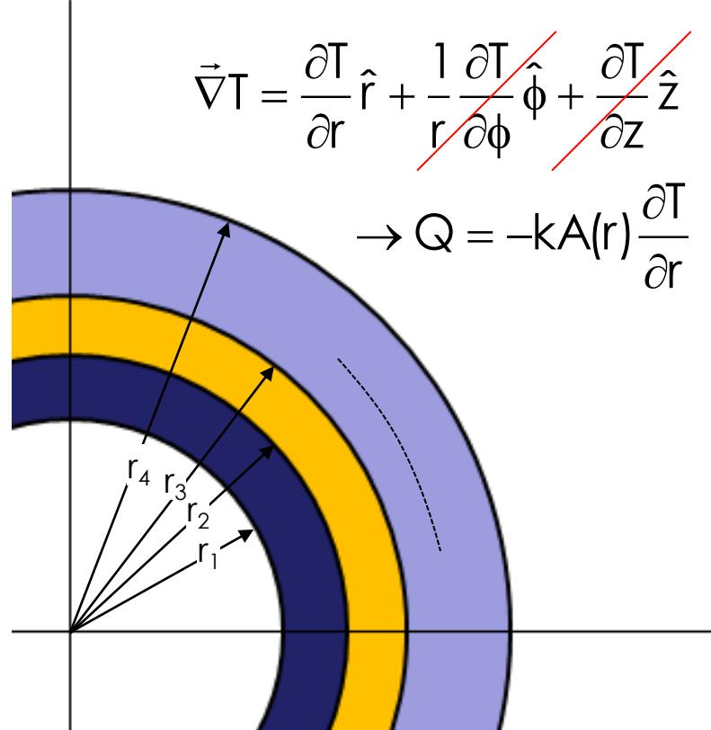
$$\frac{Q}{A(r)} = -k \frac{dT}{dr} \quad \rightarrow \int_{r_k}^{r_{k+1}} \frac{Q}{2\pi r L} dr = - \int_{T_k}^{T_{k+1}} k dT$$
