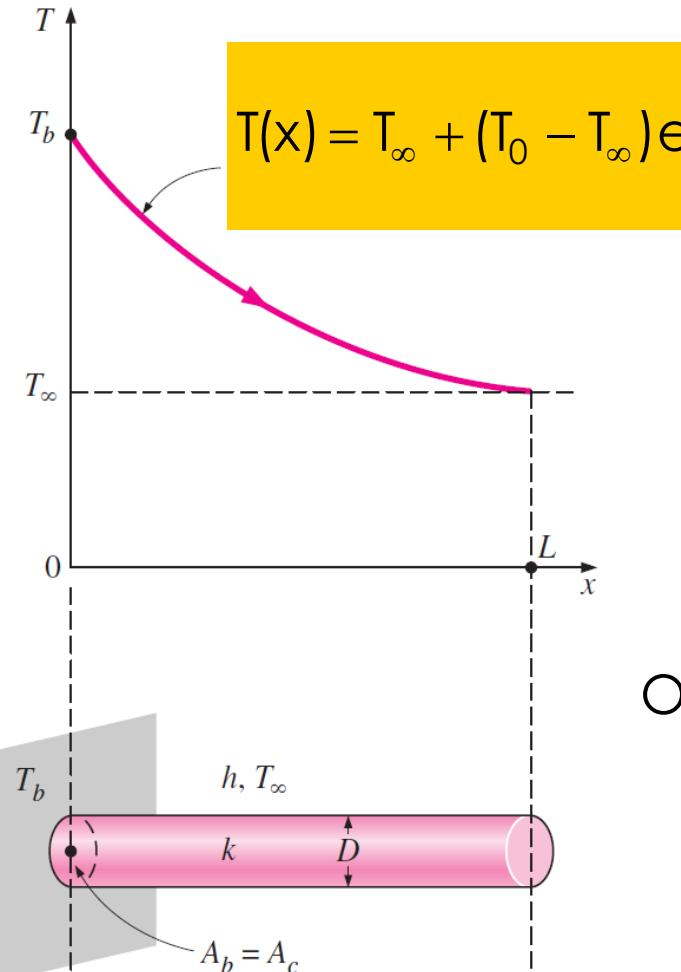
$$T(x) = T_\infty + (T_0 - T_\infty) \exp\left(-\sqrt{\frac{hp}{kA_c}} \cdot x\right)$$
