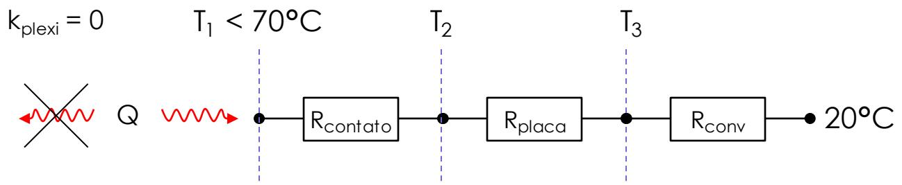
$$R_{contato} = \frac{1}{h_{contato} A} = \frac{1}{42 \frac{\text{kW}}{\text{m}^2 \text{°C}} \cdot 8 \cdot 10^{-4} \text{m}^2} = 0.030 \text{ °C/W}$$
