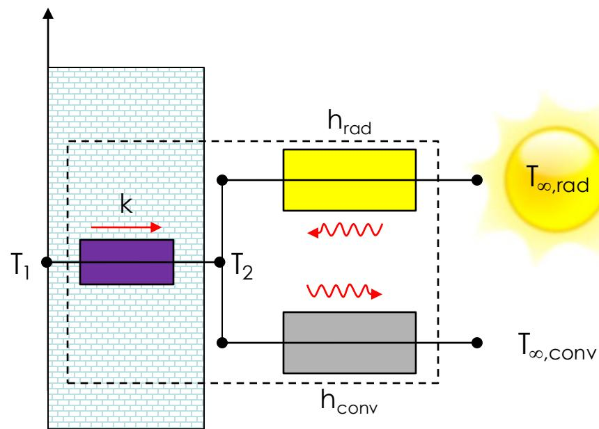
$$Q_{\text{rad}} = \frac{T_{\infty, \text{rad}} - T_2}{1/(h_{\text{rad}} A)} = \frac{T_{\infty, \text{rad}} - T_2}{R_{\text{rad}}}$$
