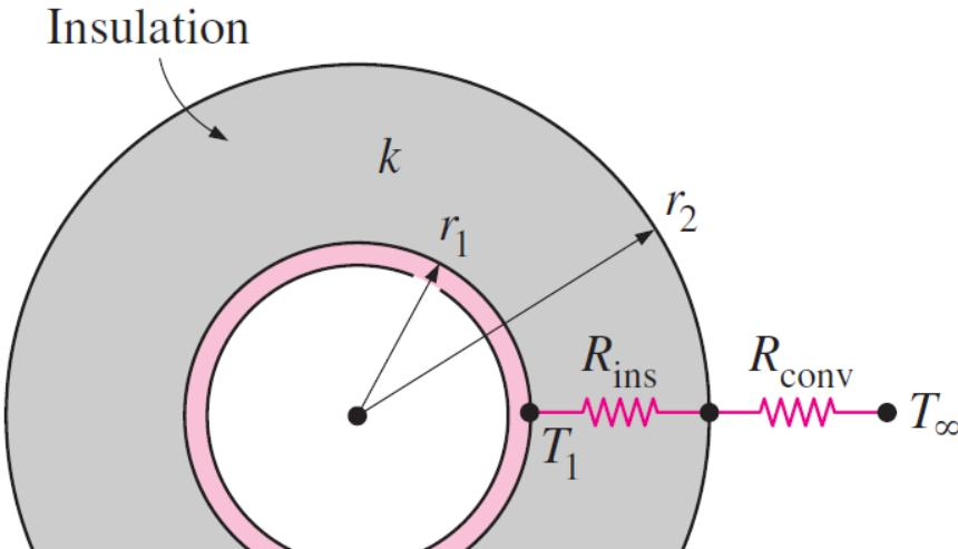
$$Q = \frac{\frac{T_1 - T_\infty}{\ln(r_2/r_1)}}{2\pi L k} + \frac{1}{h \cdot (2\pi r_2 L)}$$
