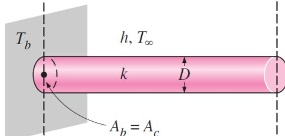
$(p = \pi D, A_c = \pi D^2/4 \text{ for a cylindrical fin})$
