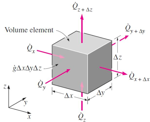
$$\frac{\partial^2 T}{\partial x^2} + \frac{\partial^2 T}{\partial y^2} + \frac{\partial^2 T}{\partial z^2} + \frac{\dot{g}}{k} = \frac{\rho C_P}{k} \frac{\partial T}{\partial t}$$
