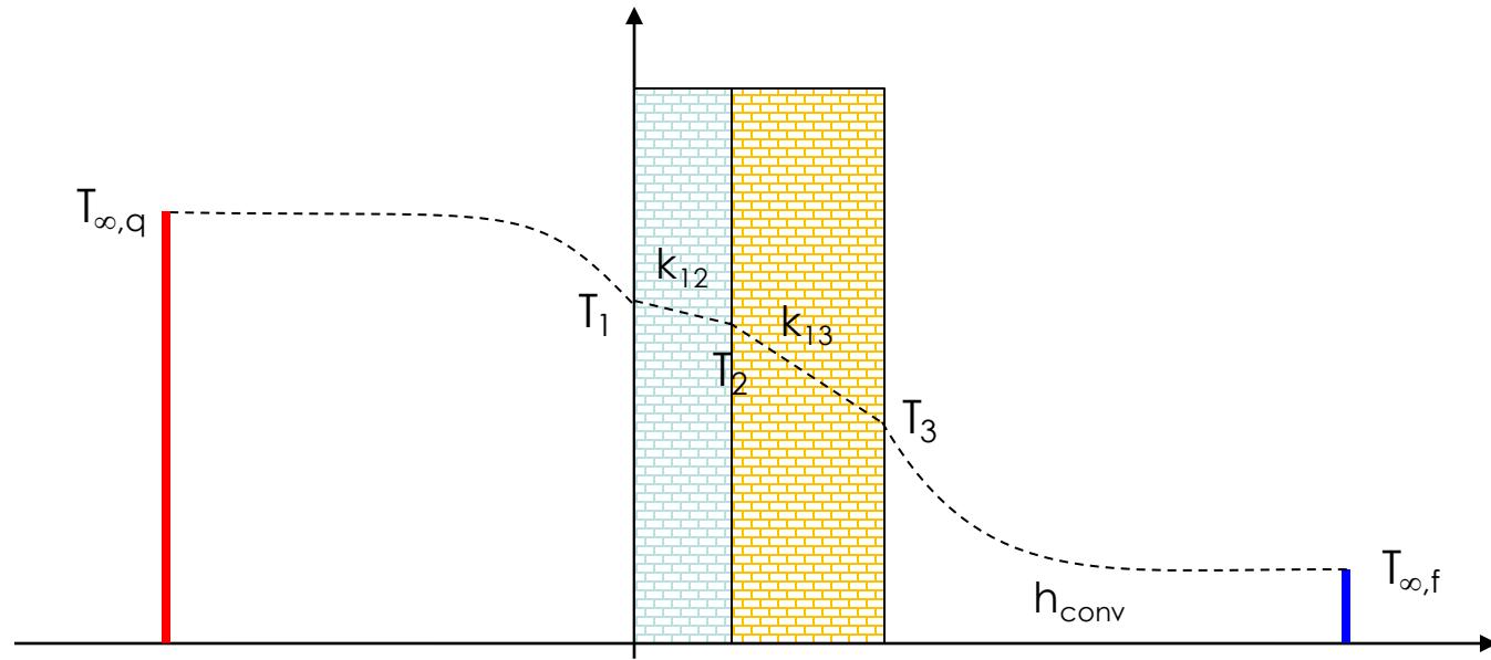
$$Q = \frac{T_{\infty,q} - T_{\infty,f}}{R_{\text{total}}} = \frac{T_{\infty,q} - T_{\infty,f}}{\underbrace{R_{\text{conv},q} + R_{\text{cond},12} + R_{\text{cond},23} + R_{\text{conv},f}}_{\sum_k R_{\text{cond},k}}}$$
