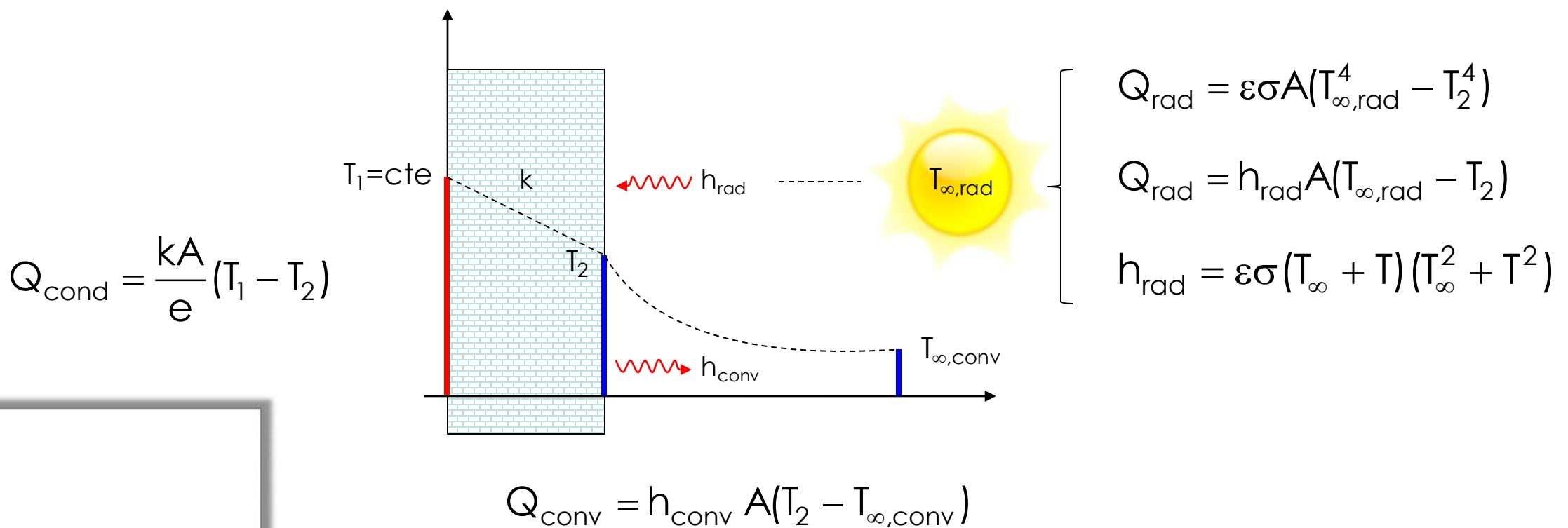
$$Q = \frac{\frac{T_q - T_f}{1 + \frac{e}{h_q A_q} + \frac{1}{k A_q} + \frac{1}{h_f A_f}}}{R_{cq} + R_{cp} + R_{cf}} \rightarrow Q = \frac{\Delta T}{R_{\text{total}}}$$
