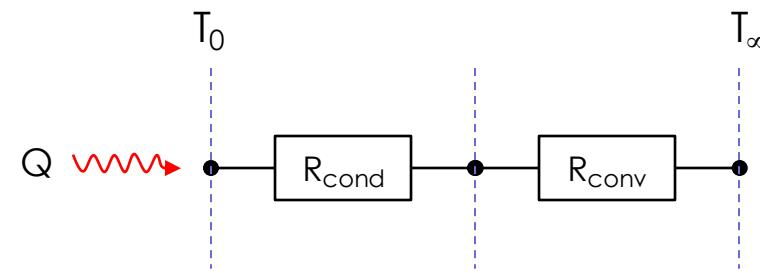
$$Q = \frac{T_{\text{sup}} - T_\infty}{\frac{L}{kA_{\text{cond}}} + \frac{1}{hA_{\text{conv}}}}$$
