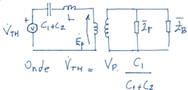
$$\text{Logo: } E_p = V_{TH} - j \left( \omega L - \frac{1}{\omega(C_1 + C_2)} \right)$$
