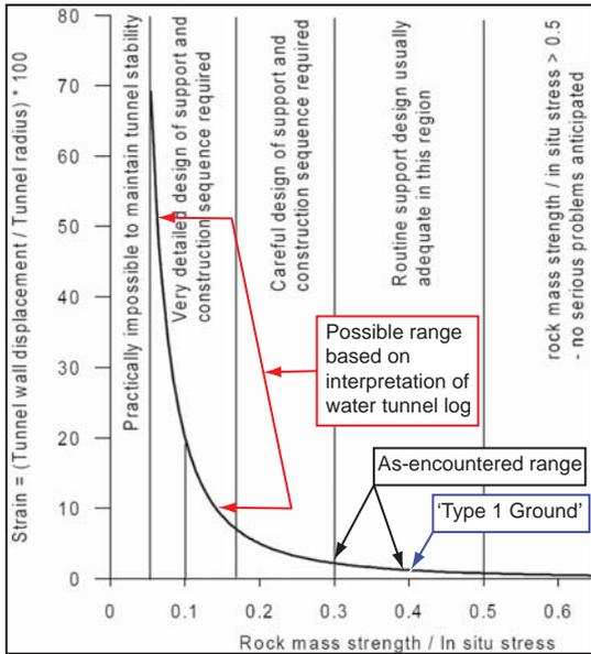
Figure 6.7.7 – Graphical representation of relative tunnelling difficulty
