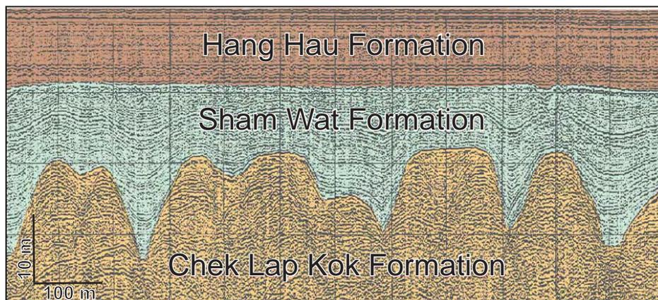
Figure 6.8.1 – Seismic boomer profile showing consolidation drapes of Sham Wat Formation sediment laid down on the gullied surface of the Chek Lap Kok Formation (Fyfe *et al.*, 2000)
