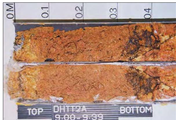
Figure 6.4.40 – Anomalous zone in saprolite interpreted as being either an infilled soil pipe or high permeability sheared zone (Koor & Campbell, 2005)
