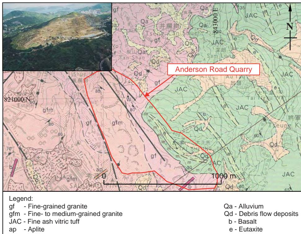
Figure 6.10.1 – Geological setting of Anderson Road Quarry
