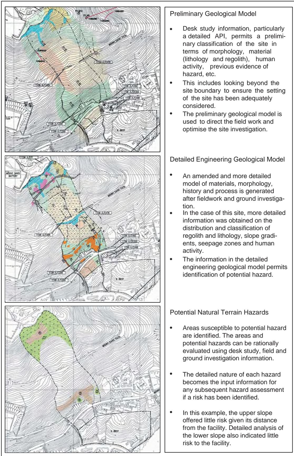
Figure 6.2.5 – Progressive development of geological models for NTHS
