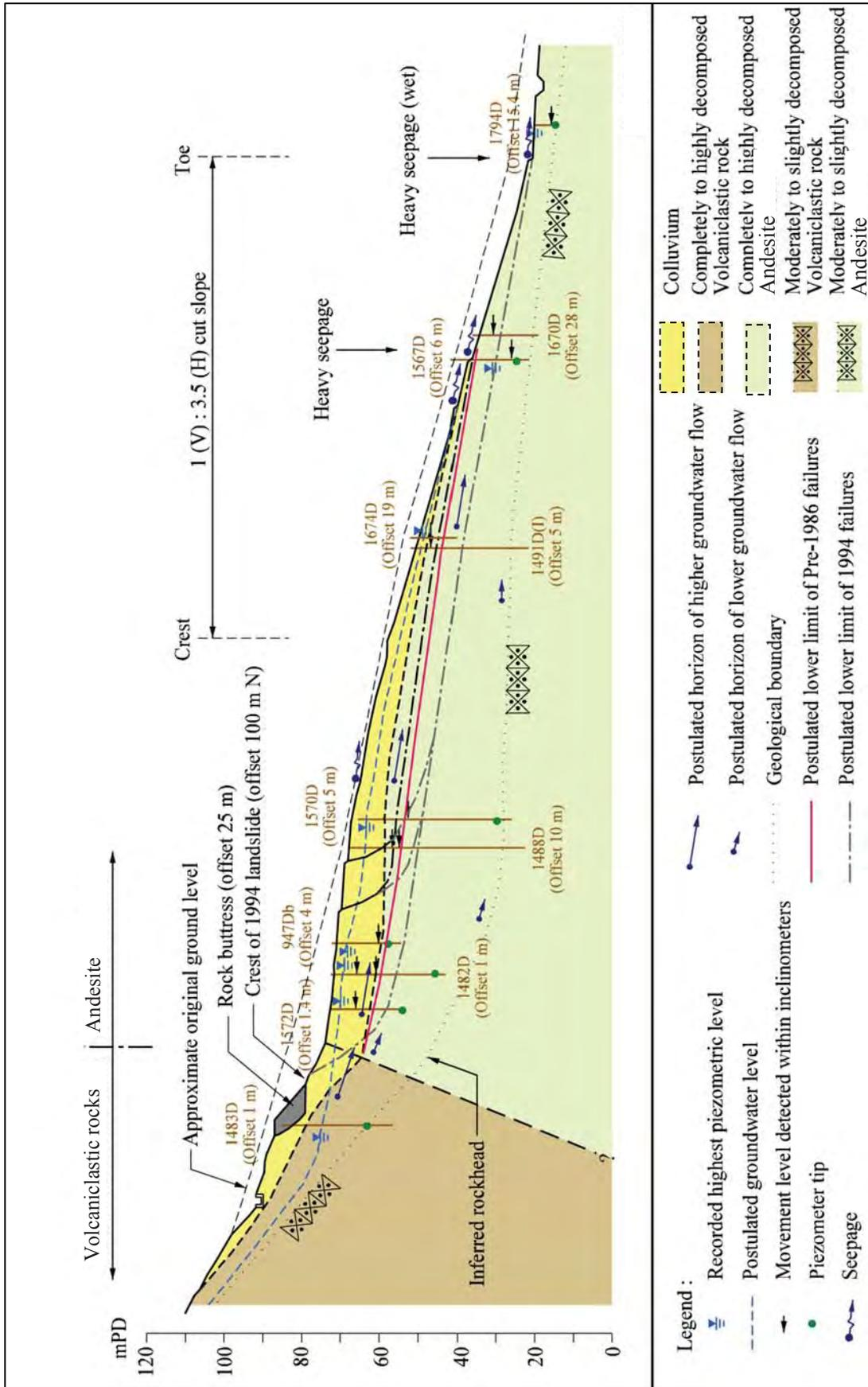
Figure 6.3.10 – Section A-A through Area 19 showing geology, deep-seated movements and high groundwater table
