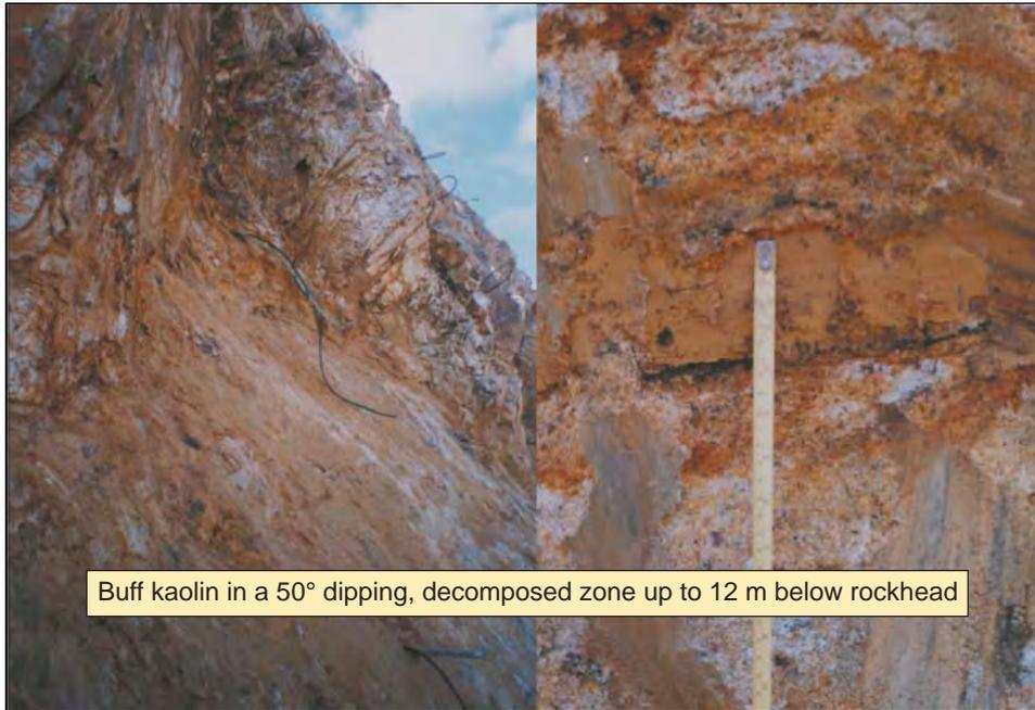
Buff kaolin in a 50° dipping, decomposed zone up to 12 m below rockhead
