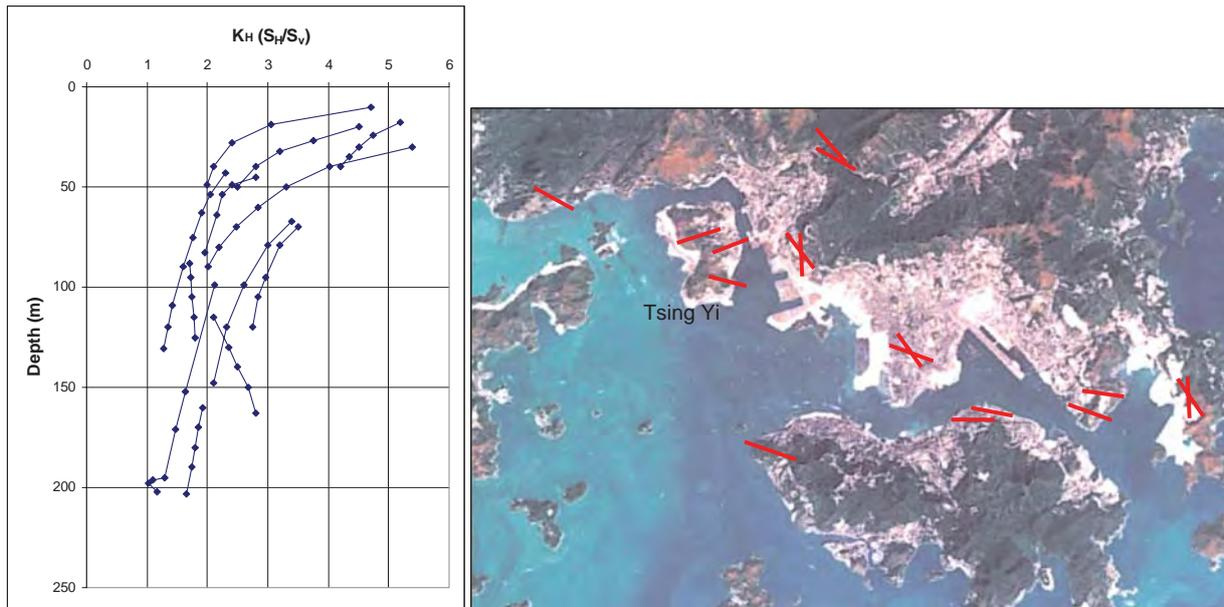
Figure 4.2.5 – Maximum horizontal stress ratio  $K_H (S_H/S_v)$  versus depth and orientations of  $S_H$  (alignment of red bars in photograph) in Hong Kong (selected data from Free *et al.*, 2000 and Route 10 investigations)
