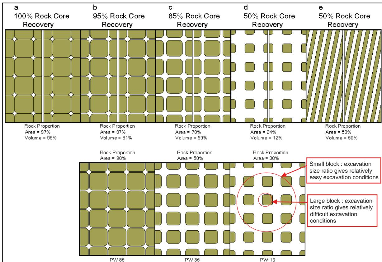
Figure 4.4.8 – Schematic depiction of rock percentage and correlation with rock core recovery (assuming recovery of 100% of the rock material). Very idealised jointing patterns and equi-dimensional blocks are shown. The percentage of rock in the ground in proportion to the percentage of rock core recovered will be larger with increasing randomness in block arrangement and increasingly poor drilling practice.
