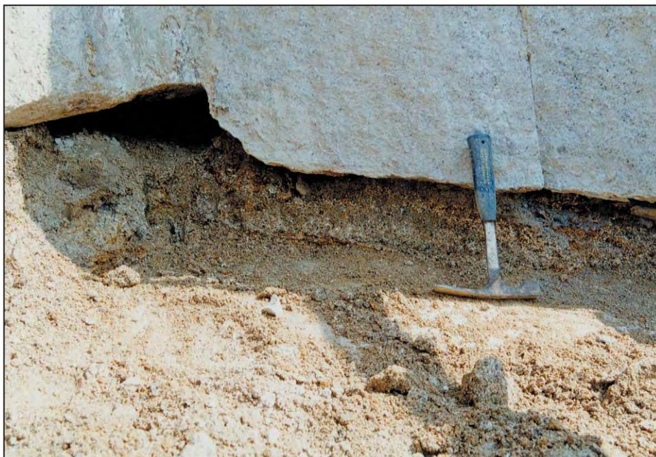
Figure 4.4.14 – Bedded granular material infilling sheeting joint
