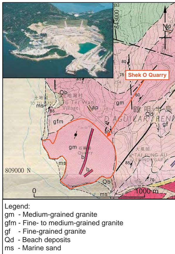
Figure 6.10.2 – Geological setting of Shek O Quarry
