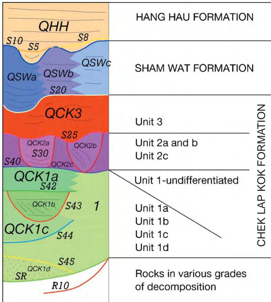
Figure 6.8.2 – Schematic relationship between the seismo-stratigraphic units and seismic reflectors at the airport reclamation site (Plant et al., 1998 after James et al., 1994 – Copyright BGS / NERC)
