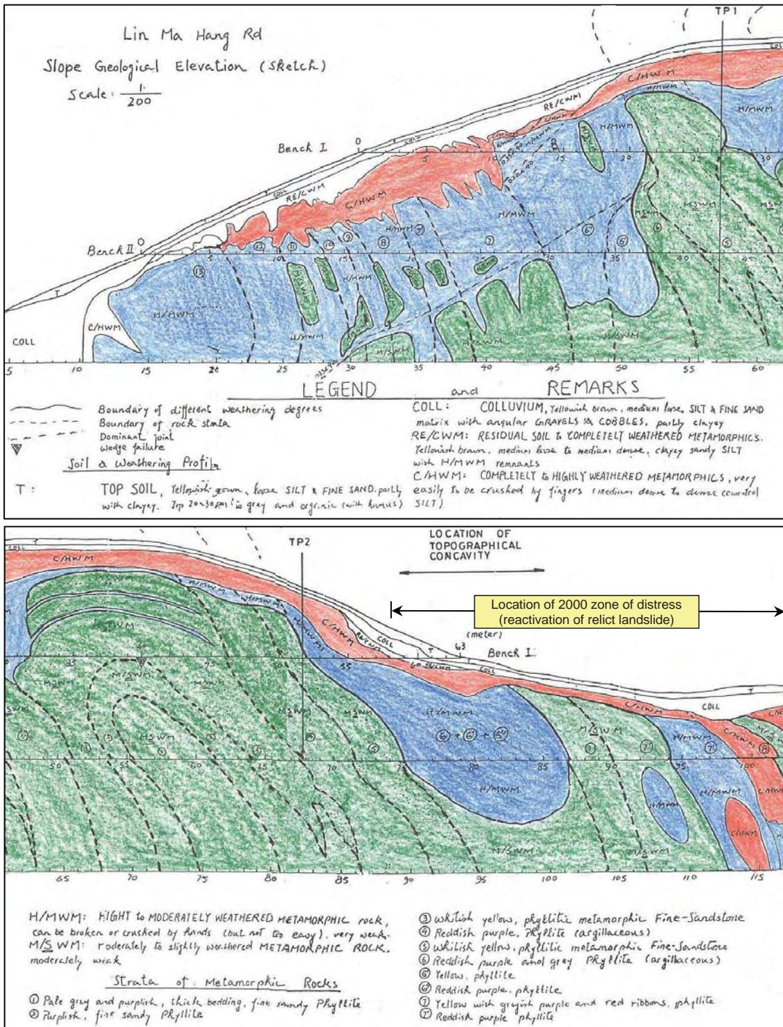
Figure 6.4.31 – Extract from the original 1981 geological face mapping record of the Lin Ma Hang Road cutting showing complex structure and weathering
