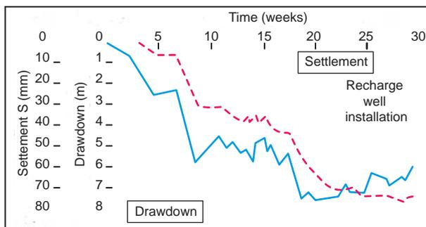
Figure 6.7.17 – Groundwater drawdown in decomposed granite and settlement recorded adjacent to Star Ferry Car Park during rock tunnelling works (after Cowland & Thorley, 1985)
