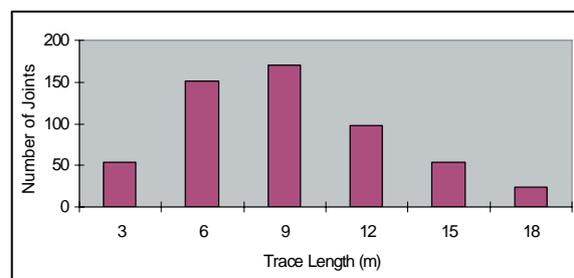
Figure 6.6.4 – Trace length distributions of joints ( $\geq 3$  m) measured in the MTRC North Point plant building and station excavations
