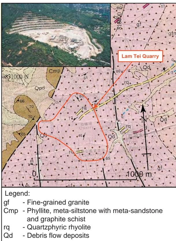
Figure 6.10.3 – Geological setting of Lam Tei Quarry
