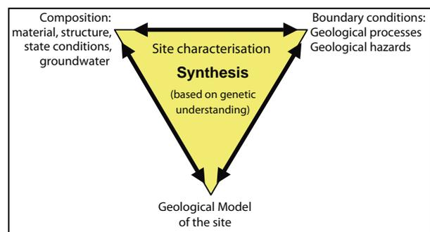
Figure 3.1.2 – Main elements of the geological model (Bock, 2006)
