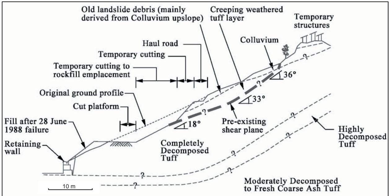
Figure 6.4.10 – Section through the 1988 landslide area at Island Road School (Irfan, 1989)
