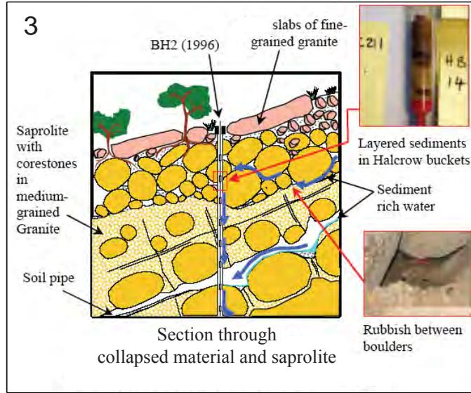
Figure 6.4.44 – Hydrogeological model for development of erosion tunnels/soil pipes at Yee King Road (after HCL, 2003a)
