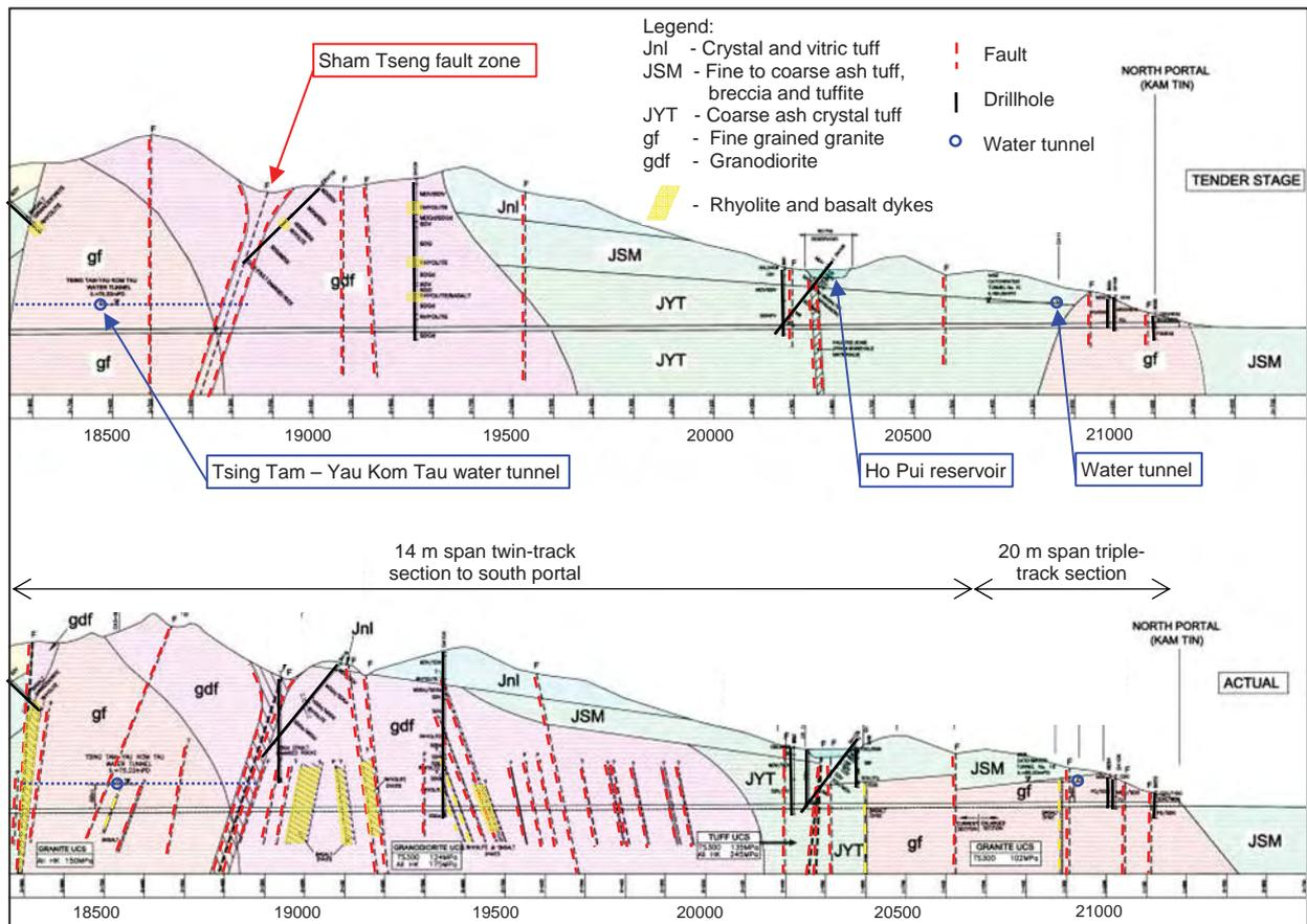
Figure 6.7.5 – West Rail Tai Lam Tunnel (northern section) – comparison of the tender design and as-built geological profiles (based on records provided by Nishimatsu-Drages Joint Venture)
