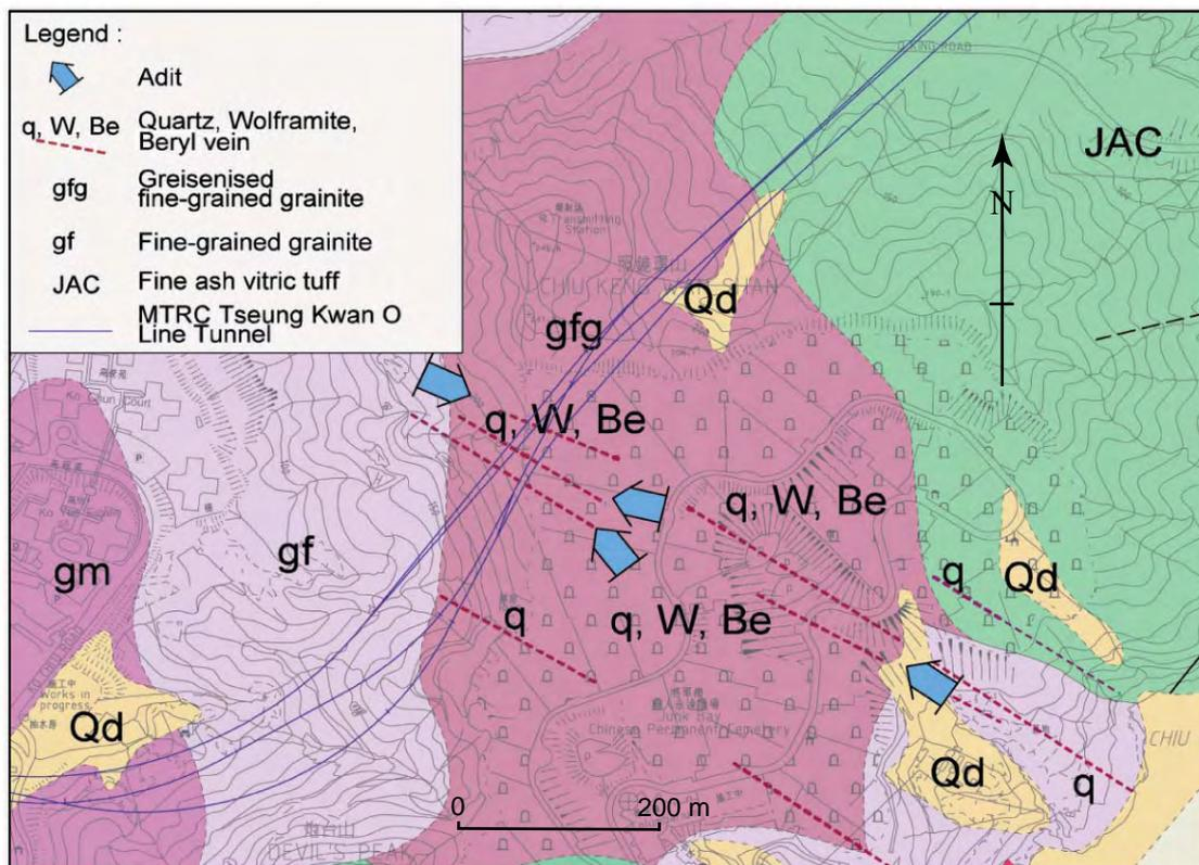
Figure 6.10.9 – Black Hill Tunnels - Extract from 1:20,000-scale geological map with mineral veins and adits associated with hydrothermal alteration highlighted
