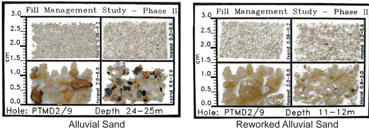
Figure 6.10.6 – Photograph of alluvial sand and reworked alluvial sand from West Po Toi marine borrow area (BCL, 1991-93)
