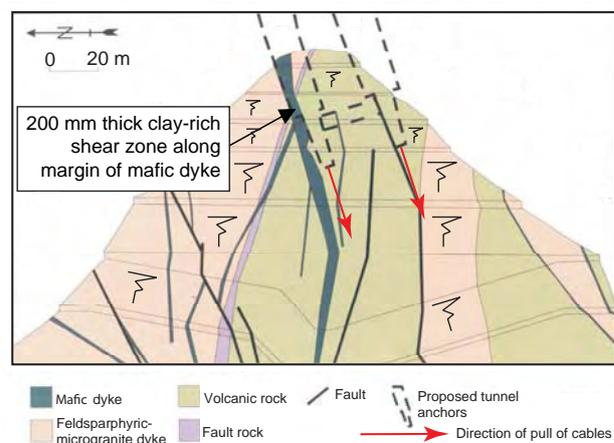
Figure 5.4.3 – Schematic geology of proposed anchorage site of the Tsing Ma suspension bridge on Tsing Yi Island (after Langford, 1991)
