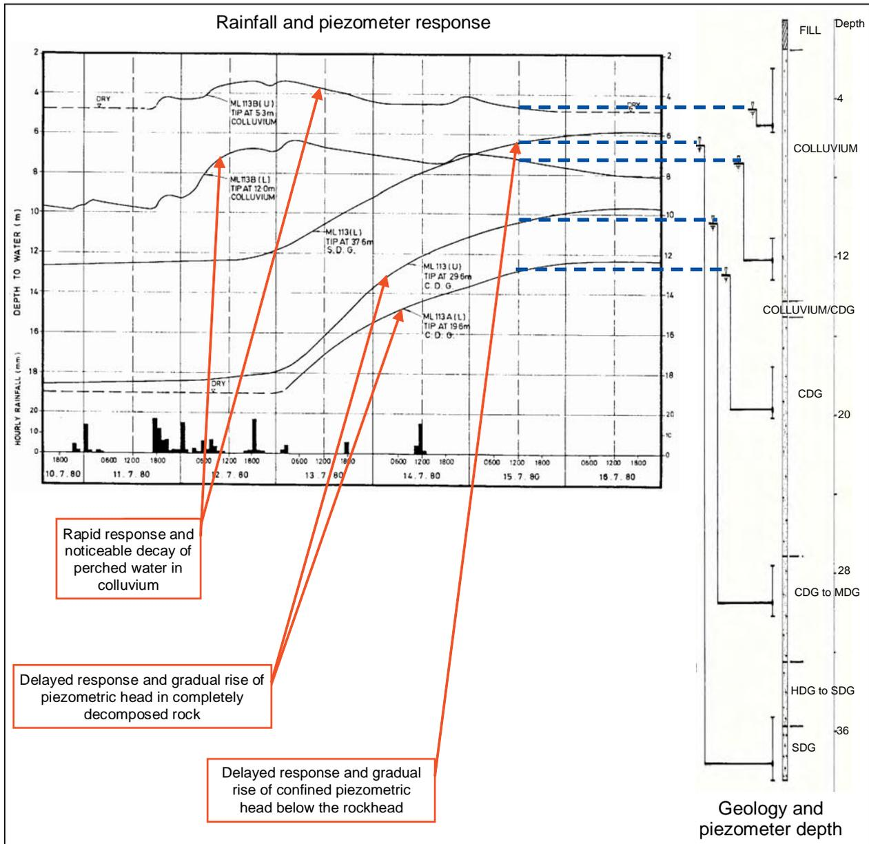
Figure 4.6.4 – Groundwater responses in colluvium and a weathered granite profile in the Mid-levels study area of Hong Kong Island (after GCO, 1982)
