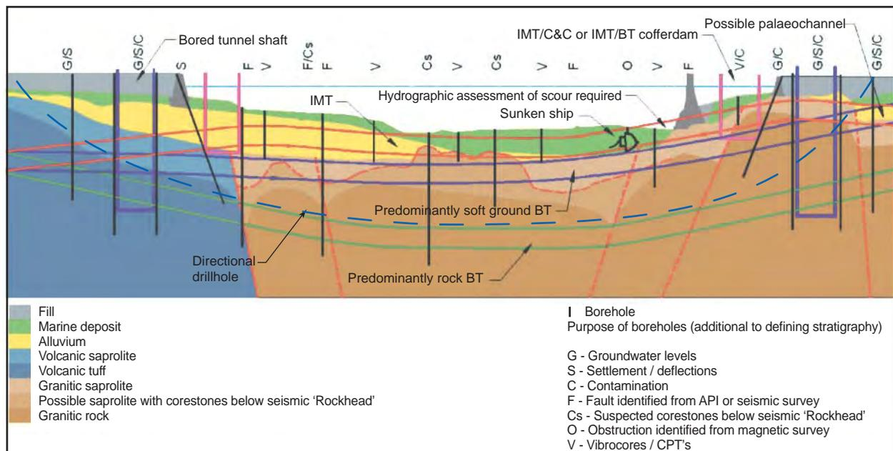
Figure 6.7.15 – Typical layout of investigations for a marine tunnel crossing
