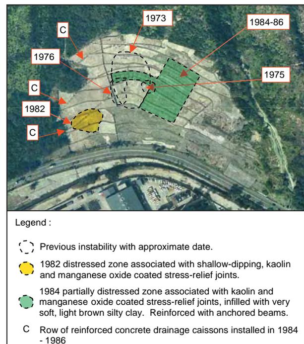
Figure 6.4.16 – 2003 Orthophoto of the ‘Pepco’ slope near Nam Wan, South Tsing Yi showing previous distressed zones
