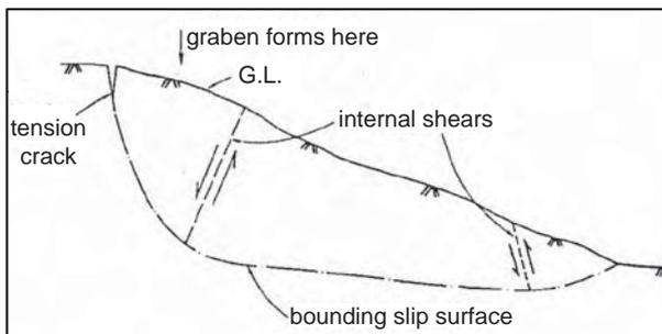
Figure 3.5.4 – Typical internal shears required to permit movement in a non-circular slide (Hutchinson, 1987)
