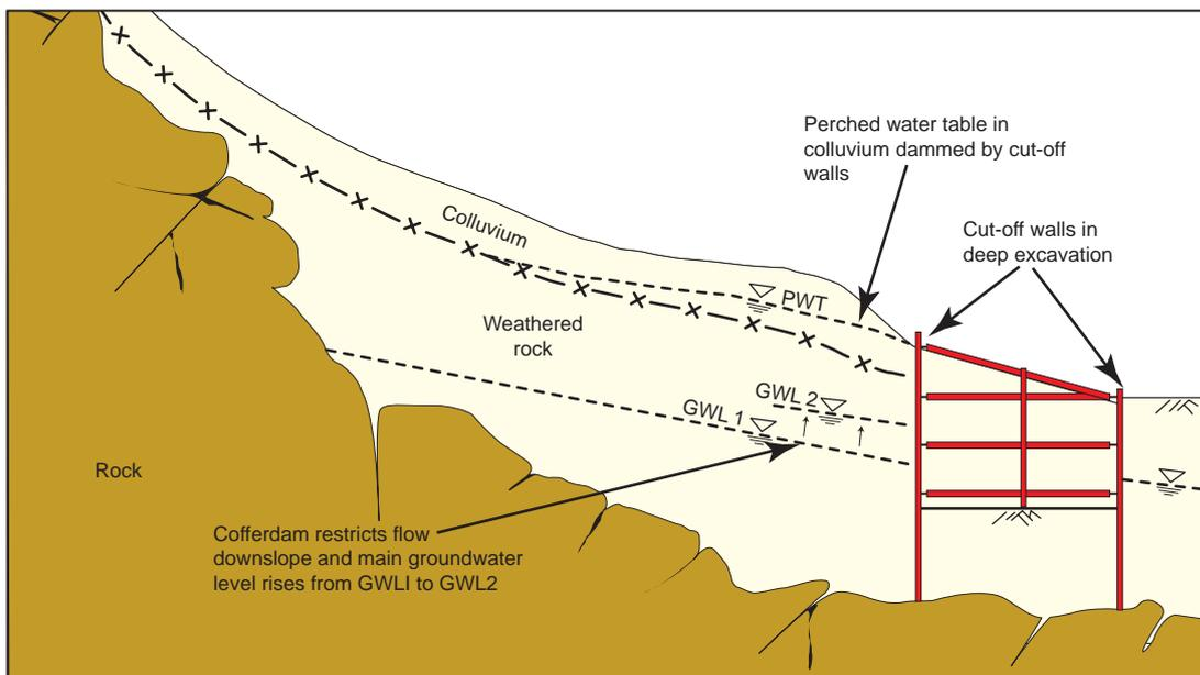
Figure 6.6.7 – Groundwater damming on hillsides due to deep excavations
