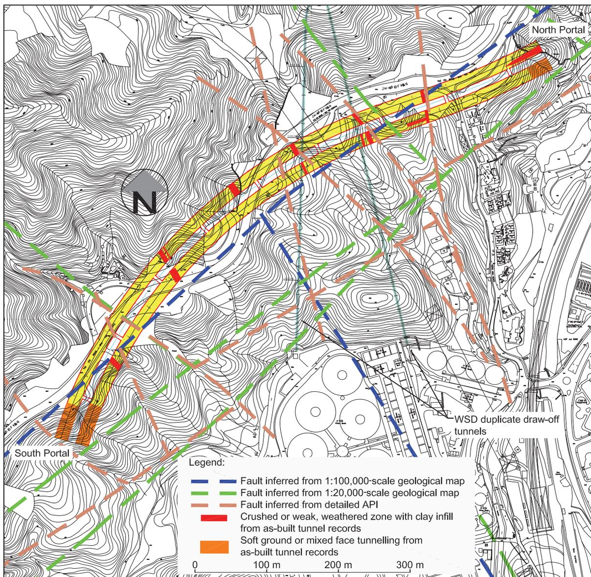
Figure 6.7.3 – Layout plan of geological structures encountered in the Sha Tin Heights tunnel and faults and photolineaments inferred from detailed API and the 1:20,000-scale (GCO, 1986a) and 1:100,000-scale (Sewell *et al.*, 2000) published geological maps
