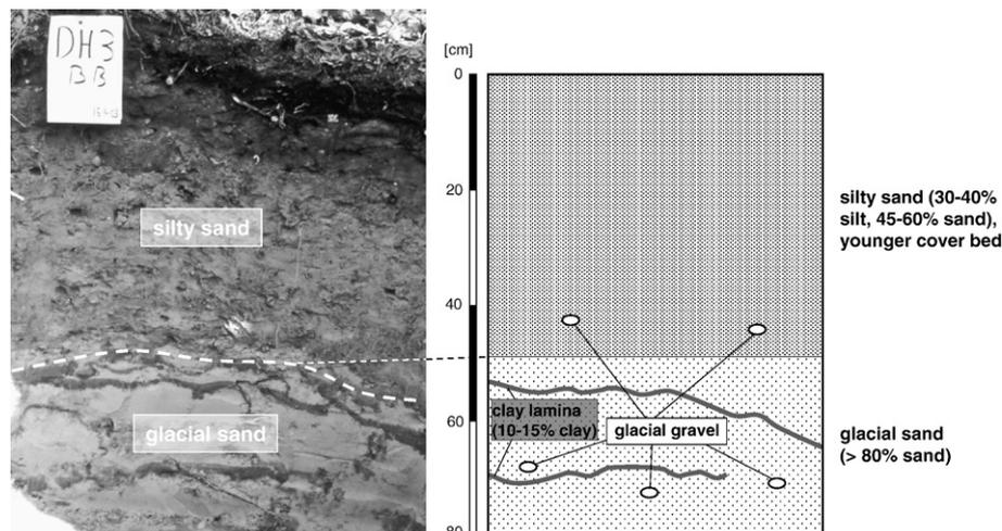
Fig. 6. Soil profile with sandy-silty mantle covering glacial sands in the Dahleener Heide. The upper cover bed is assumed to be of eolian origin with relic cryoturbation features (late Pleistocene) and subsequent Holocene pedogenesis. The clay bands in the subsoil may be older soil formations or of geologic origin.
