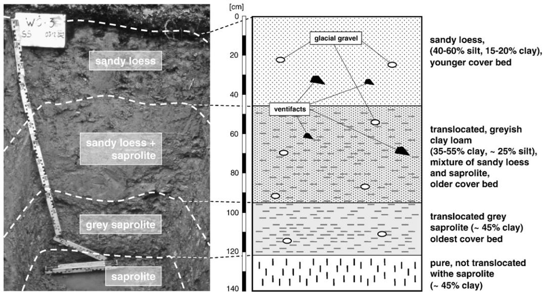
**Fig. 7.** Soil profile with silt mixed and transported material, and *in situ* saprolite in the Wermsdorfer Forst. The upper cover bed is of high silt content (sandy loess). The base of the soil profile is saprolite derived from rhyolite. The mixed glacial gravels in the soliflucted saprolite demonstrate its movement. The intermediate cover bed is a mixture of residual material and sandy loess.
