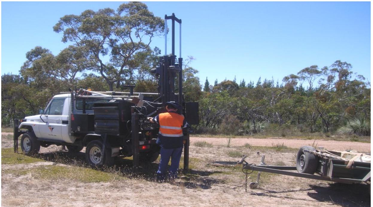
*The push core drilling rig used to measure regolith depth in the Adelaide Hills, South Australia. A combination of existing site data, new drilling and field measurements (e.g. road cuttings and gullies) were used to develop a predictive model of weathering depth in the region.*
