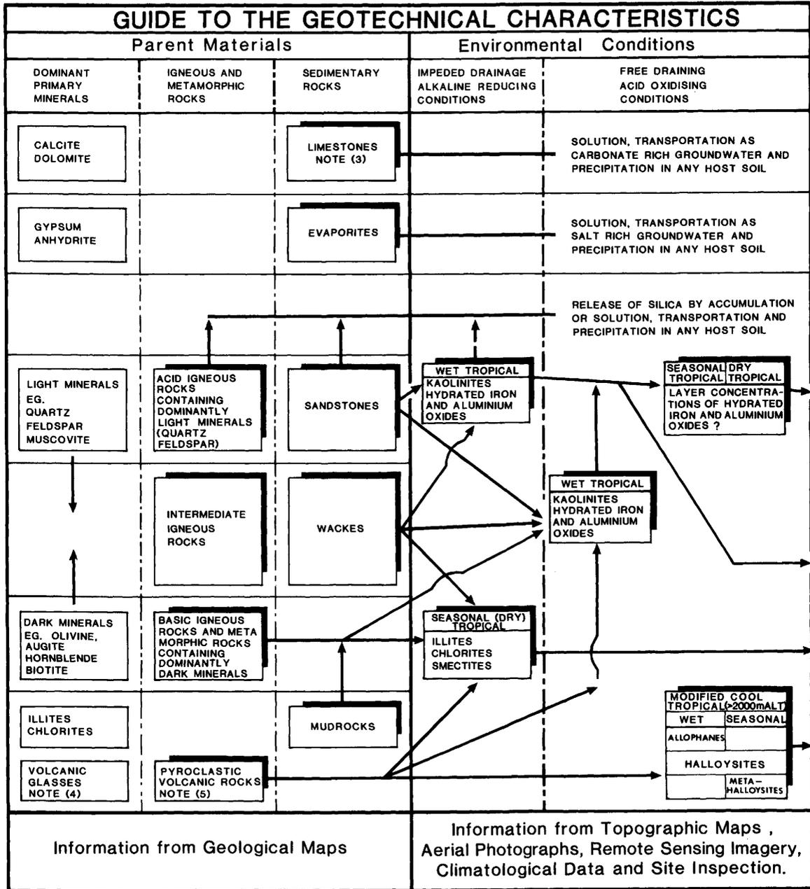
FIG. 3.2. Guide to the geotechnical characteristics of tropical residual soils.
