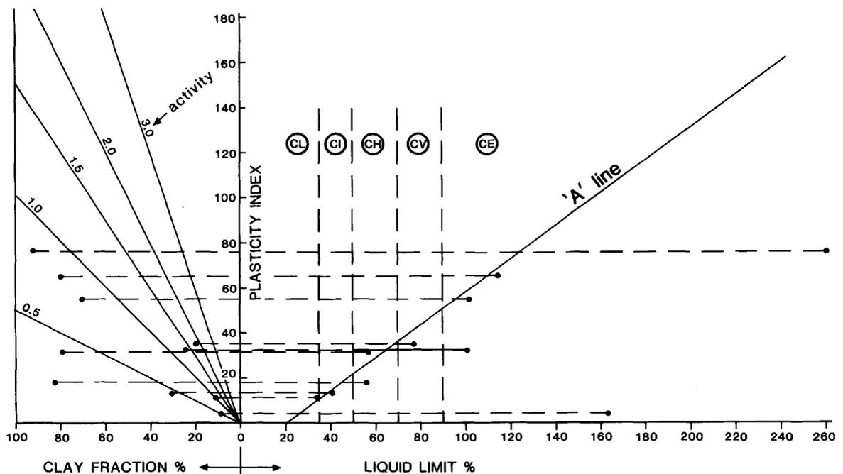
FIG. 5.2. Examples of classification by plasticity and clay fraction.
