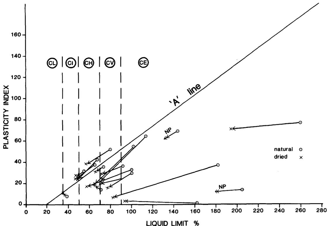
FIG. 5.1. Effect of drying on plasticity for some examples of tropical residual soils.
