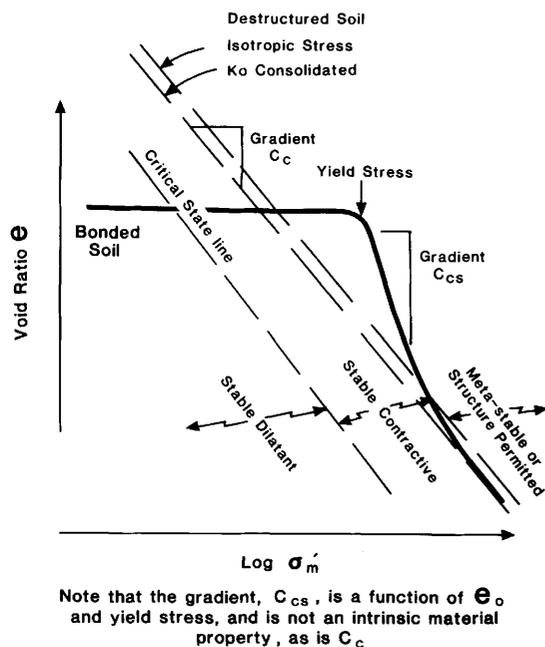
FIG. 6.5. Stress-void ratio state of a residual soil related to the states possible for the de-structured soil. Note that the gradient,  $C_{CS}$  is a function of  $E_0$  and yield stress, and is not an intrinsic material property, as is  $C_c$ .
