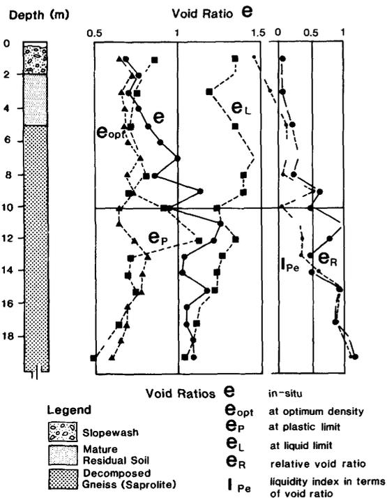
FIG. 6.7. Profile of weathered gneiss at Guri Dam, Venezuela, plotted in terms of void ratio (after Prusza *et al.* 1983).
