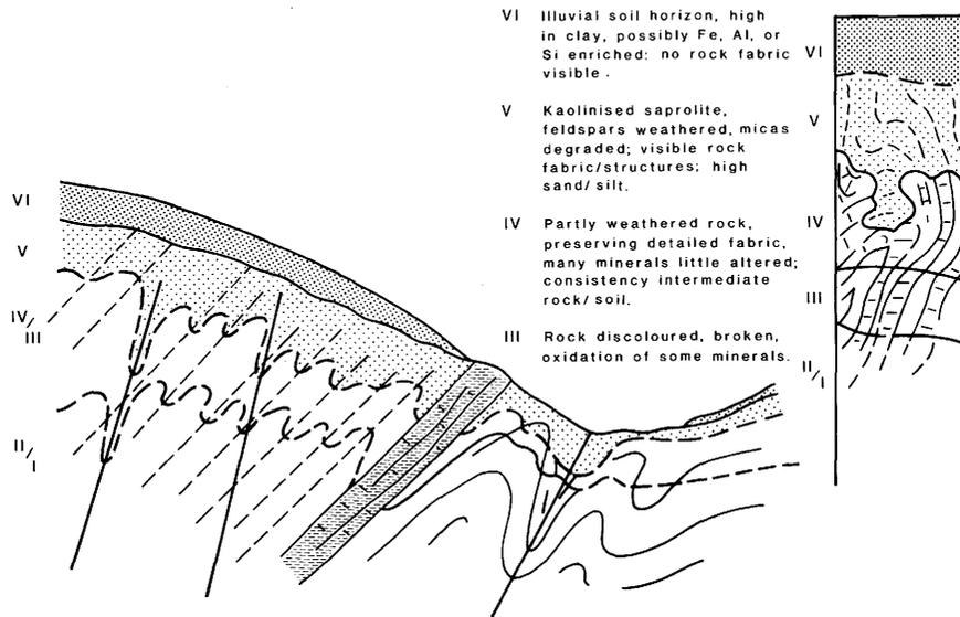
FIG. 2.7. Transect of weathering depths and profile characteristics over banded metamorphic rocks (adapted from Deere & Patton 1971).
