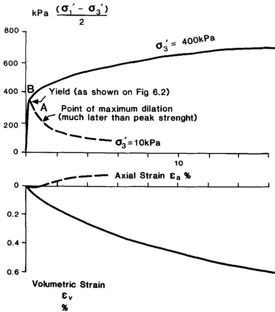
FIG. 6.3. Drained triaxial tests on residual soil from basalt.
