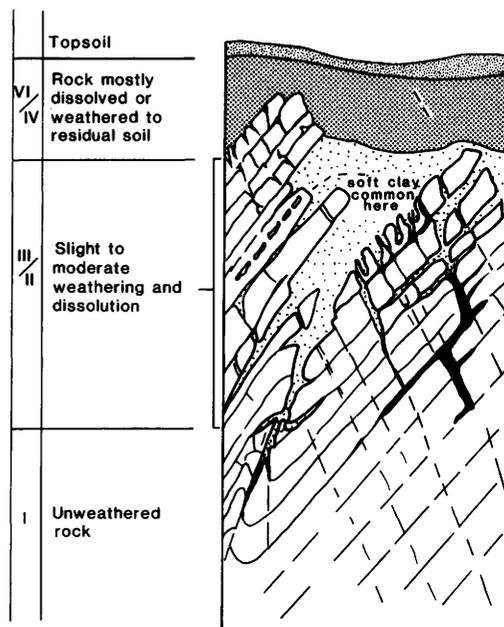
FIG. 2.6. Typical weathering profile for carbonate rocks. The occurrence of a saprolite Zone (V) is restricted to impure (silty/sandy) carbonates, while Zone IV characteristics occur mainly in chalky limestones. Soft clays often occur as cavity fillings and are not strictly in situ (adapted from Deere & Patton 1971).
