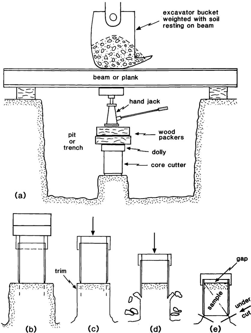
FIG. 5.9. Jacking undisturbed core-cutter sampler.
