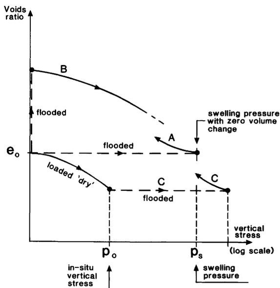
FIG. 5.6. Measurement of swelling characteristics of expansive clays.
