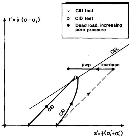
FIG. 5.5. Failure of residual soils with bonding, following different stress paths.
