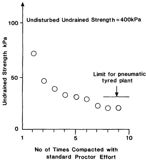
FIG. 6.9. Effect of repeated laboratory compaction on undrained strength of porous residual soil from basalt (Mauritius).
