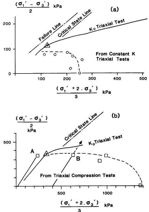
FIG. 6.2. Yield stresses observed in tests on residual soils; (a) residual soil from gneiss (Sandroni, 1981); (b) residual soil from basalt (Vaughan *et al.* 1988).
