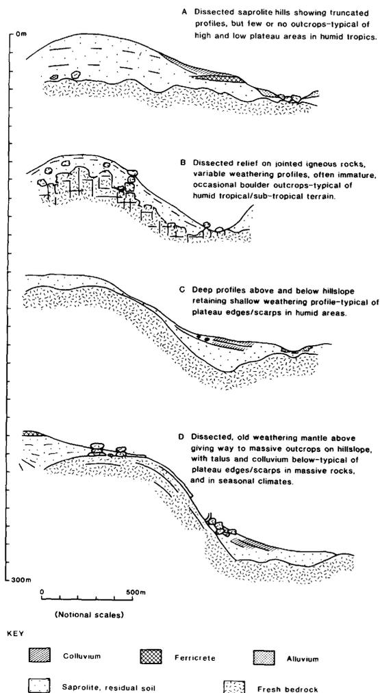
FIG. 2.10. Examples of hillslope profiles illustrating common sequences of weathering and landforms.
