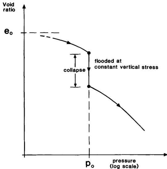
FIG. 5.7. Behaviour of a collapsing soil.
