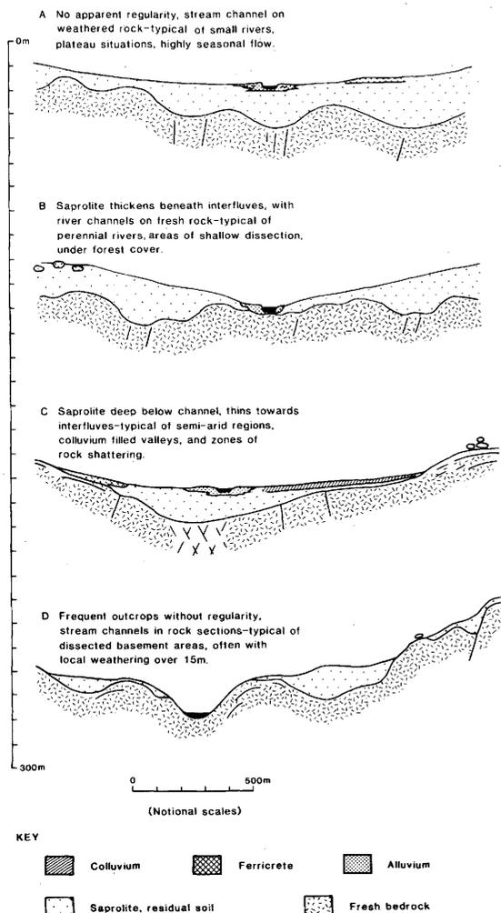
FIG. 2.9. Examples of transverse valley profiles illustrating common patterns of variation in weathering depths.
