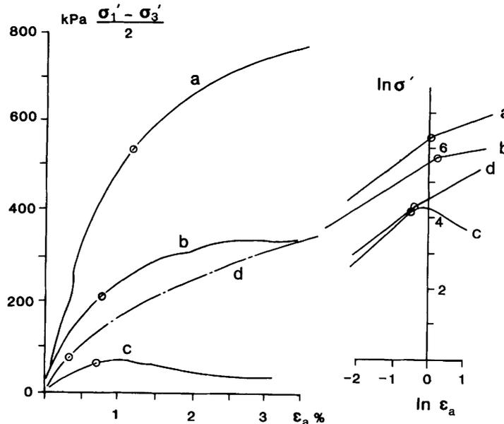
FIG. 6.4. Yield in laboratory triaxial tests shown by plots at natural and log-log scales. (a)–(c) Drained compression tests on soil from basalt. (d) Constant stress ratio tests,  $K = 0.45$ , on soil from gneiss (after Vaughan 1988).
