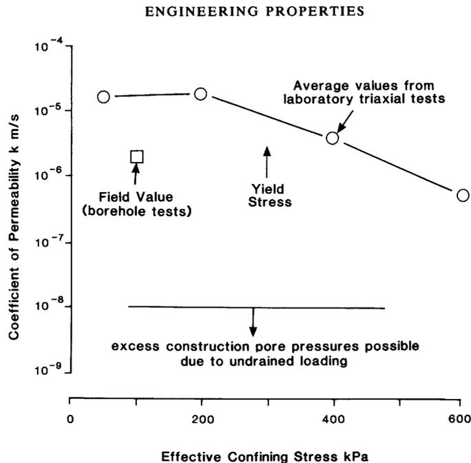
FIG. 6.8. Variation of permeability with confining stress: residual soil from gneiss at Guri Dam (after Medina & Liu 1982).
