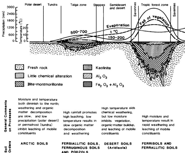
FIG. 2.2. Diagram of relative depth of weathering and weathering products as they relate to some environmental factors in a transect from the Equator to the north polar regions (after Strakhov 1967).
