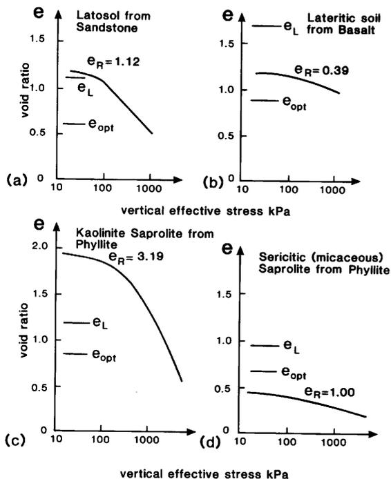
FIG. 5.3. Examples of void ratio used as an index (after Vaughan *et al.* 1988).
