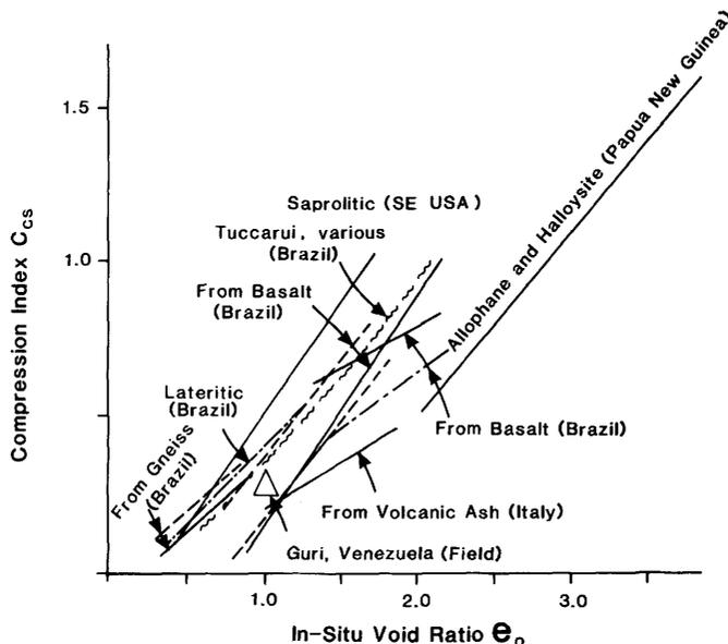
FIG. 6.6. Relationships between compression index,  $C_{cs}$ , and initial void ratio,  $e_0$  (after Wallace 1973; Lacorda *et al.* 1985).
