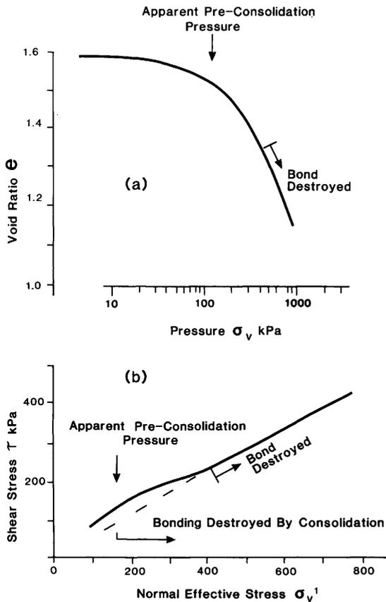
FIG. 6.1. Apparent pre-consolidation pressure (Vargas 1973); (a) observed in the oedometer; (b) influence on drained shear strength in direct shear.
