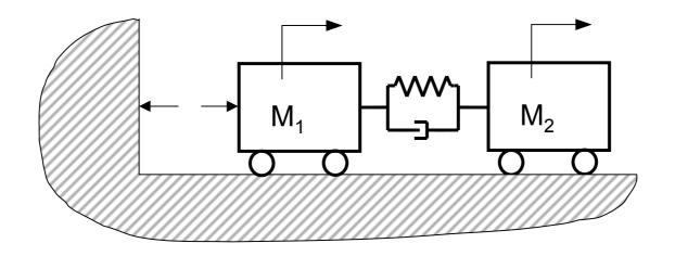
Positioning the load  $M_2$  (while using  $x_1$  for feedback):
