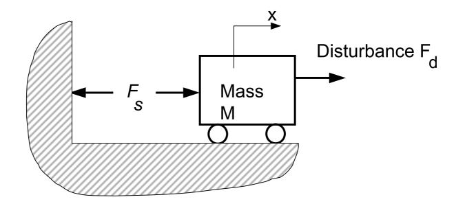
Slide: mass = 5 kg Required accuracy 10  $\mu$ m at all times Disturbance (f.e. friction) = 3 N
