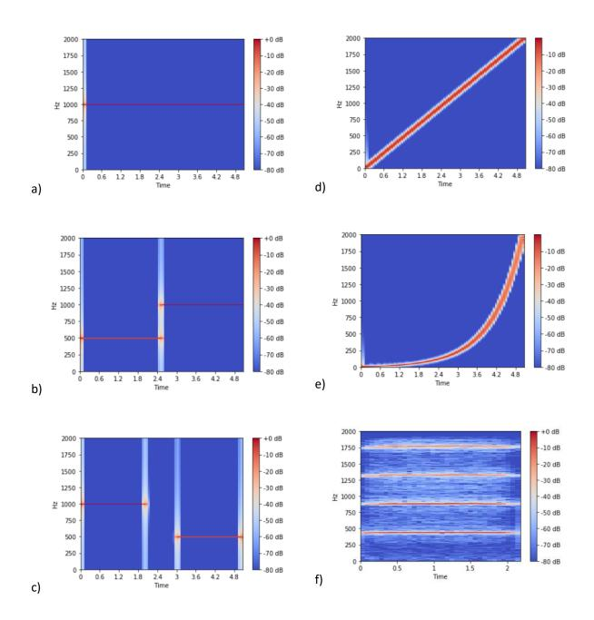
1 – Draw (sketch) the corresponding waveforms of the following spectrograms.
