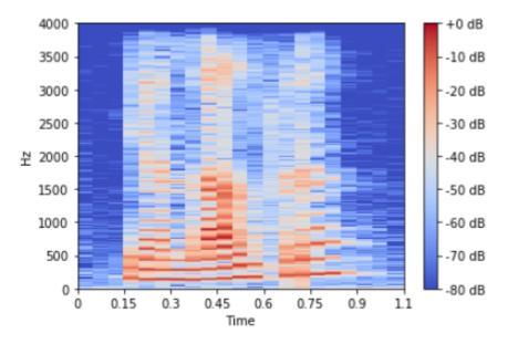
3 – The following figure is a zoom-in of the above spectrogram. Calculate the frequency resolution and the window size (in samples)?
