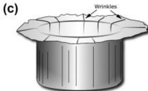
Defect in drawn cup due to wrinkling
