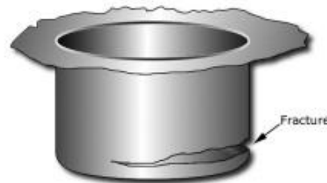
Failure of cup by fracturing during drawing
