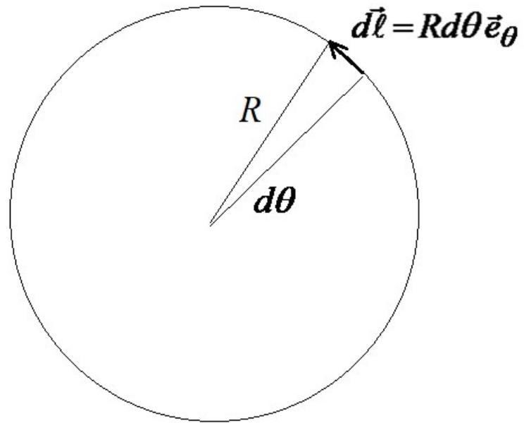
$$\Gamma_C = \oint_C \vec{V} \cdot d\vec{\ell} = \int_0^{2\pi} \frac{\Gamma}{2\pi R} \vec{e}_\theta \cdot R d\theta \vec{e}_\theta = \int_0^{2\pi} \frac{\Gamma}{2\pi} d\theta = \Gamma$$
