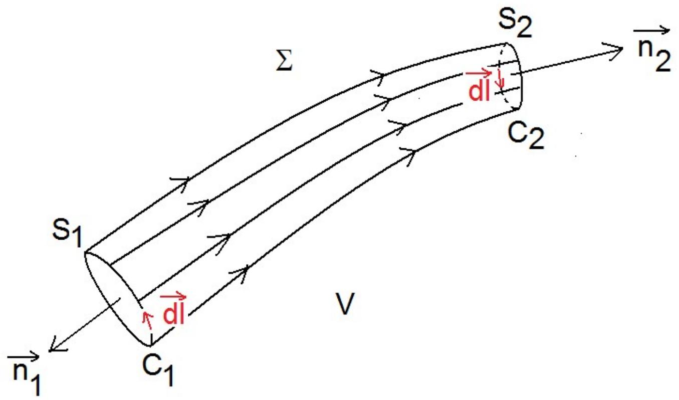
$$\int_S \vec{\omega} \cdot \vec{n} dA = \int_{S_1} \vec{\omega} \cdot \vec{n}_1 dA + \int_{S_2} \vec{\omega} \cdot \vec{n}_2 dA = 0 \quad (2.2)$$
