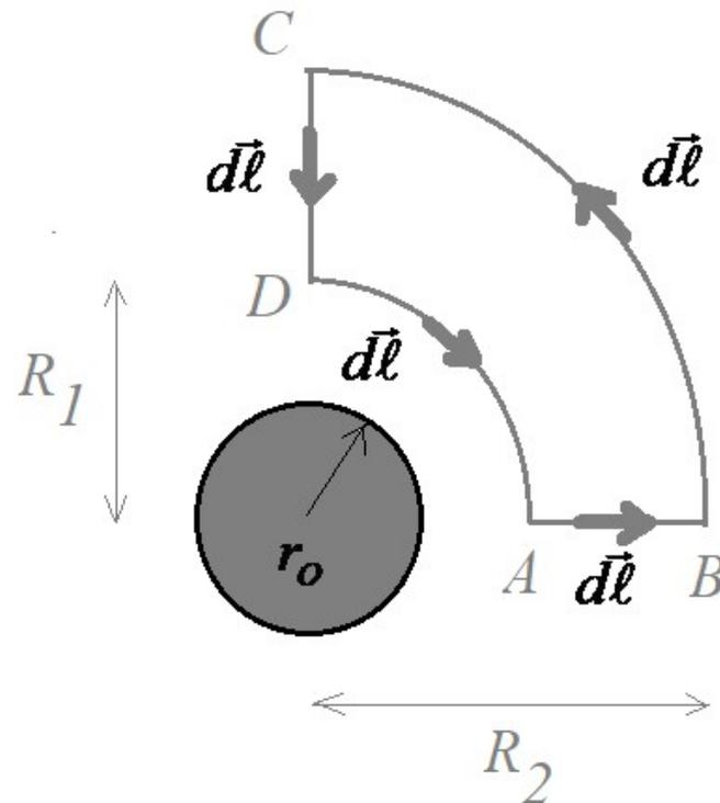
$$\Gamma_C = \oint_C \vec{V} \cdot d\vec{\ell} = \int_{AB} \vec{V} \cdot d\vec{\ell} + \int_{BC} \vec{V} \cdot d\vec{\ell} + \int_{CD} \vec{V} \cdot d\vec{\ell} + \int_{DA} \vec{V} \cdot d\vec{\ell}$$
