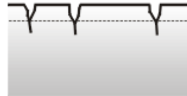
C. Corrosion fatigue cracks have little branching
