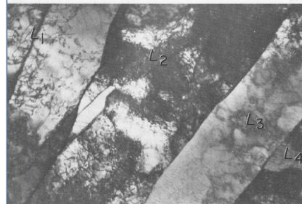
Thin-foil specimen 26,000× 3278 Thin-foil electron micrograph of the 0.03 C, 2 Mn alloy steel specimen in micrograph 3276, showing dislocation substructure in four of the martensite laths (marked L_1 to L_4 ).
