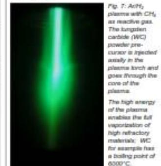
Fig. 7: Ar/H<sub>2</sub> plasma with CH<sub>4</sub> as reactive gas. The tungsten carbide (WC) powder precursor is injected axially in the plasma torch and goes through the core of the plasma.
