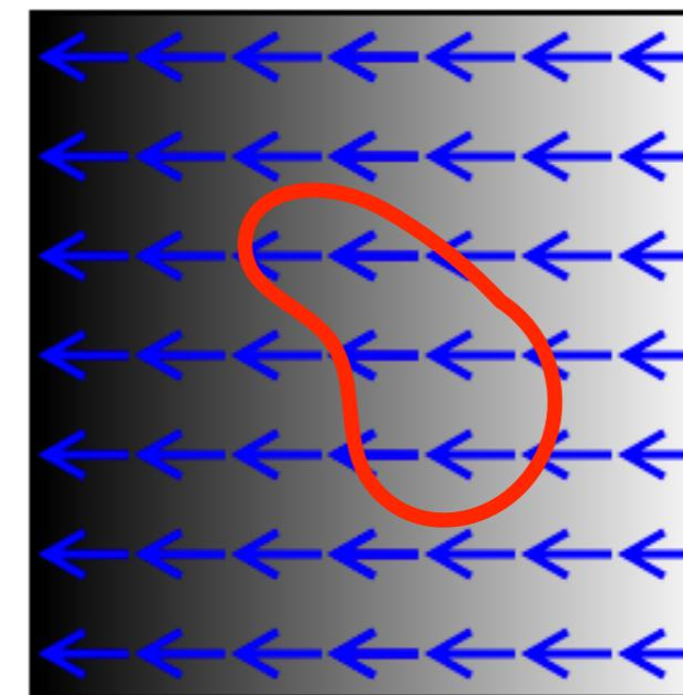
$$\frac{\partial Q}{\partial t} = \frac{\partial}{\partial t} \int_V u \, dV = \int_V \frac{\partial u}{\partial t} dV = - \oint_S \vec{\phi} \cdot \vec{n} dS$$
