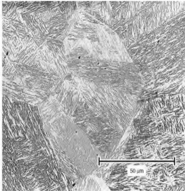
**Fig. 9.15** Lath martensite in water-quenched low-alloy steel. 2% nital etch. Original magnification 500× Source: Ref 9.6
