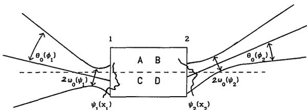
Fig. 1. Optical paraxial system illuminated by an arbitrary beam  $\Psi_1(x_1)$ . The  $ABCD$  matrix elements are real,  $\Psi_2(x_2)$  is the output beam, and  $\theta_0(\phi_1)$ ,  $\theta_0(\phi_2)$ ,  $\omega_0(\Psi_1)$ , and  $\omega_0(\Psi_2)$  are the divergences and minimum widths of the input and output beams, respectively.
