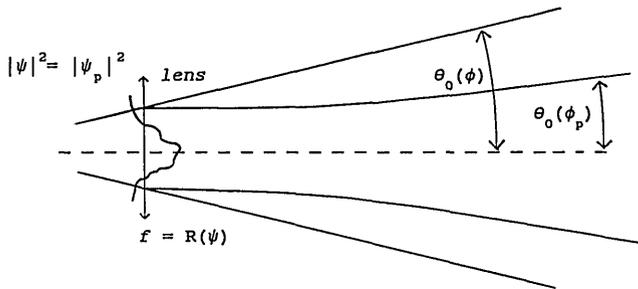
Fig. 2. Divergence  $\theta_0(\phi)$  of the beam  $\Psi(x)$  and divergence  $\theta_0(\phi_p)$  of the collimated beam  $\Psi_p(x)$ . An on-axis and nontilted beam is depicted for clarity.
