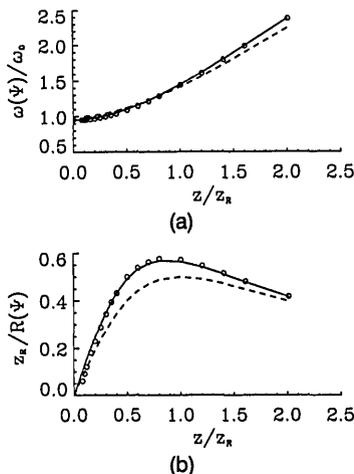
Fig. 4. Evolution of the (a) width and (b) radius of curvature of the diffracted Gaussian beam:  $\omega_0$  is the width of the input Gaussian beam and  $z_R$  is its Rayleigh range. The open circles are numerical data, based on the Fresnel integral, with a 99.4% criterion; the solid curve is the *ABCD* law prediction; the dashed curve is the evolution of the nondiffracted Gaussian beam.
