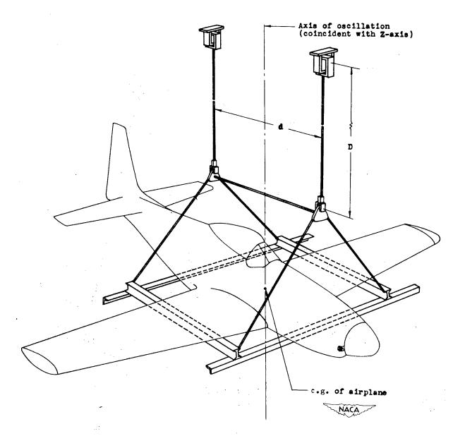
Figure 3.- Airplane and swinging gear arranged for the determination of the moment of inertia about the Z-axis by the bifilar torsion pendulum method.
