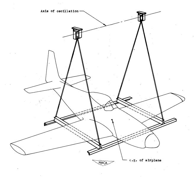
Figure 2.- Airplane and swinging gear arranged for the determination of the moment of inertia about the Y-axis by the compound-pendulum method.
