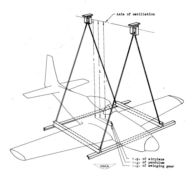
Figure 1.- Airplane and swinging gear arranged for the determination of the moment of inertia about the X-axis by the compound-pendulum method.
