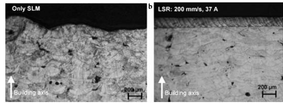
Fig. 41. Cross section of a surface created using SLM only (left) and SLM plus laser re-melting (right). Adapted from [362].
