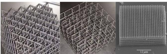
**Fig. 26.** AM lattices: octet truss lattice (left, [31]) and square lattice (center, [31]) produced using SLM, and photonic crystal with a micro woodpile structure made using two-photon polymerization (right, [247]).
