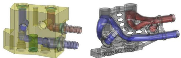
**Fig. 12.** Solid model of a water redistribution manifold redesigned for AM: original design made in PEEK with perpendicular drilled channels (left) and optimized version printed in titanium (right). The redesign reduced turbulence induced vibration forces by 90%. Images courtesy of ASML.
