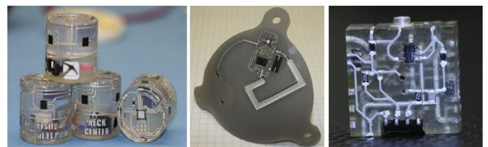
Fig. 34. Examples of AM objects with integrated electronics produced using a combination of stereolithography and direct print technologies [193] (left and center) [195] (right).
