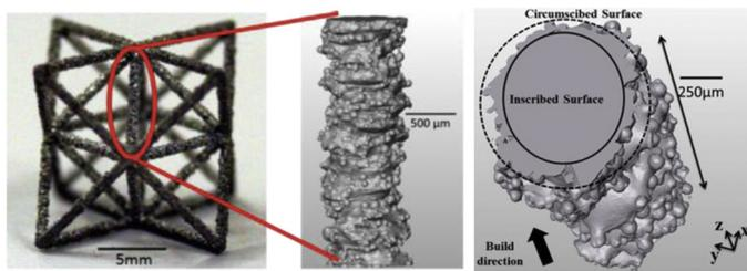
Fig. 39. EBM octet-truss unit cell (left), 3D reconstruction of a 1 mm strut from X-ray tomography (center), and an isometric view of the strut showing the diameter variation by the inscribed and circumscribed diameters (right). Adapted from [314]. Note that the strut exhibits surface roughness at length scales associated with the layering and with the powder.
