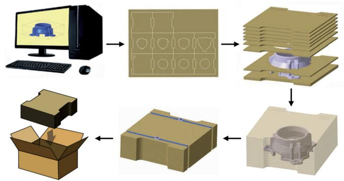
Fig. 21. Schematic of the Pack & Strat<sup>®</sup> process. Adapted from [34].
