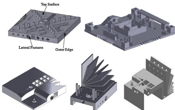
Fig. 46. AM benchmarks with design related features from [239] (top left), [196] (top right), [180] (bottom left), [63] (bottom center), and [363] (bottom right). Adapted from [239,363].
