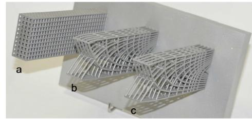
**Fig. 27.** Beams with lattice structures produced by SLM: periodic structure (a, left), flux of force adapted structure (b, center), and flux of force adapted structure with straightened struts (c, right) [324].
