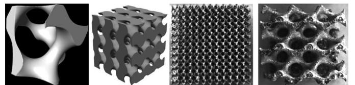
**Fig. 29.** Schoen Gyroid as a unit cell (left), volume generated from Schoen Gyroid unit cells (center left), Schoen Gyroid cellular structure with a 15% volume fraction and unit cell size of 2 mm (center right), and with a unit cell size of 8 mm (right). Both samples produced by SLM [140].
