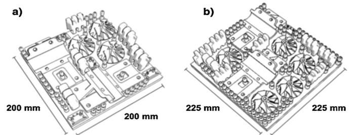
**Fig. 51.** The build platform and printed parts used for the cost calculations in [38]: EBM layout (left, a) and DMLS layout (right, b).
