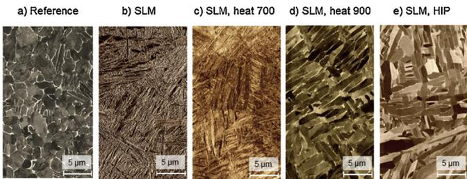
**Fig. 23.** SEM micrographs of etched surfaces showing the different grain structures of as-wrought (a) and SLM TiAl6V4 (b) with post heat treatment at 700 °C (c), 900 °C (d), or hot isostatic pressing (e). Adapted from [164].
