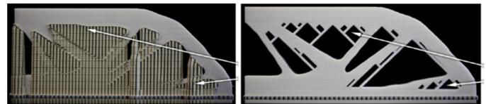
Fig. 42. Topology optimized cantilever beam successfully built with support (left) and redesigned to be self-supporting (right). Arrows indicate where build failures occur if no support strategy is implemented. Adapted from [185].
