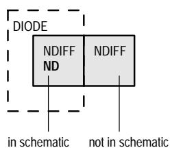
**Note:** ND is only intended for simulation of reverse leakage currents and junction capacitances. It is not recommended to use this diode as an active circuit element.
