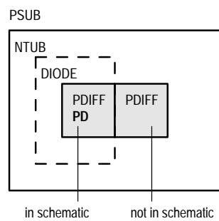
Note: PD is only intended for simulation of reverse leakage currents and junction capacitances. It is not recommended to use this diode as an active circuit element.
