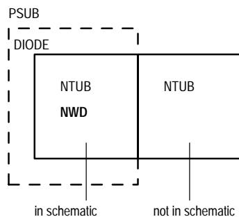
Note: NWD is only intended for simulation of reverse leakage currents and junction capacitances. It is not recommended to use this diode as an active circuit element.
