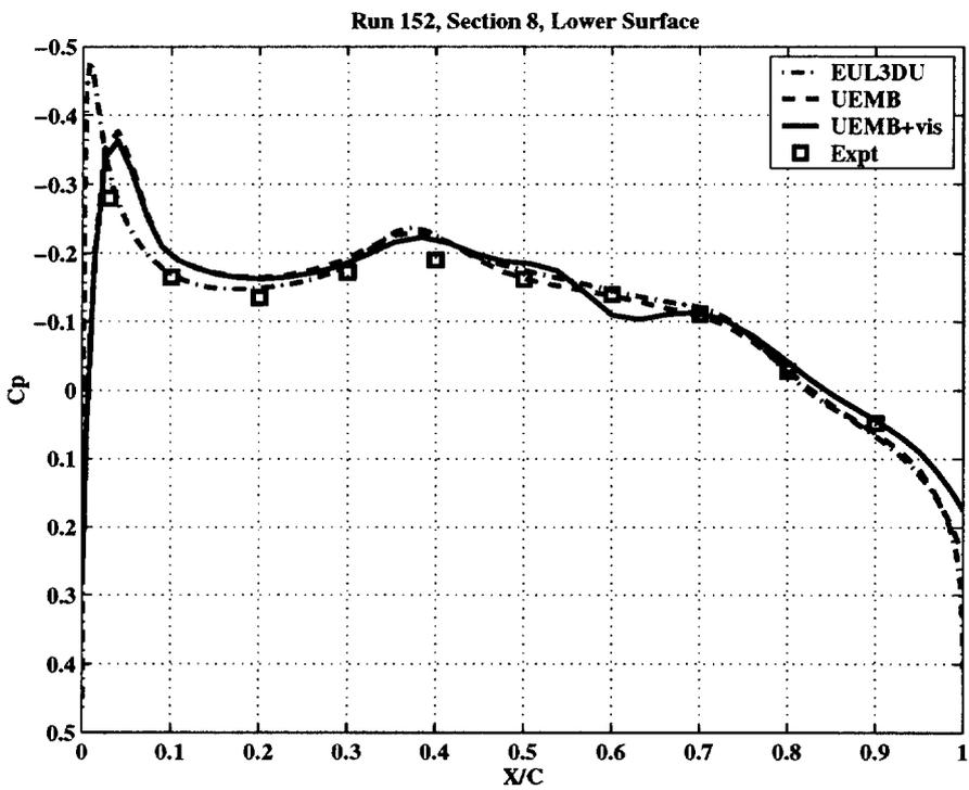
Figure 2 Comparison of EUL3DU and UEMB at section 8 for run 152. Cp is plotted for a) upper surface, and b) lower surface. This figure shows that different tip modelling has less effect than other factors (such as inclusion of viscosity, designated UEMB+vis)
