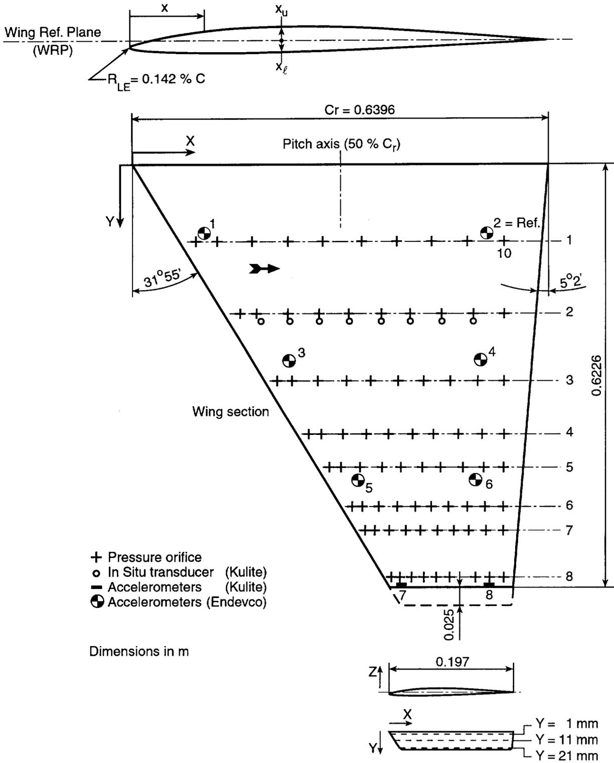
Figure 1: NLR F-5 clean wing, location of pressure orifices and transducers
