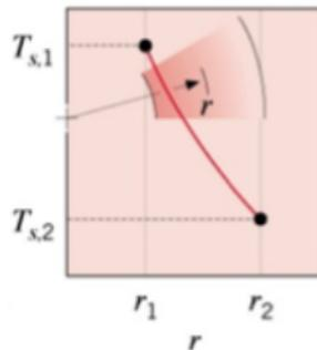
$$q_r = \frac{2\pi Lk}{\ln(r_2/r_1)} (T_{s,1} - T_{s,2})$$
