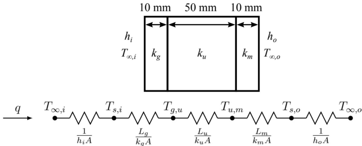
$$q_x = \frac{T_{\infty,i} - T_{\infty,o}}{\left(\frac{1}{h_i} + \frac{L_g}{k_g} + \frac{L_u}{k_u} + \frac{L_m}{k_m} + \frac{1}{h_o}\right) \frac{1}{A}} = \frac{20 - (-15)}{\left(\frac{1}{5} + \frac{0,01}{0,17} + \frac{0,05}{0,026} + \frac{0,01}{0,12} + \frac{1}{15}\right) \frac{1}{1}}$$
