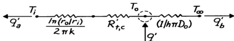
$$q' = q'_a + q'_b \Rightarrow q' = \frac{T_o - T_i}{\frac{\ln(r_o/r_i)}{2\pi r} + R'_{t,c}} + \frac{T_o - T_\infty}{\frac{1}{h\pi D_o}}$$
