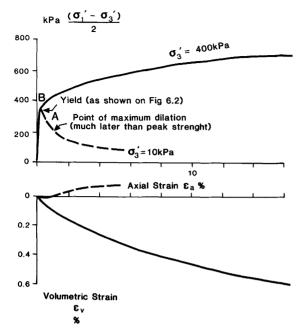
Fig. 6.3. Drained triaxial tests on residual soil from basalt.
