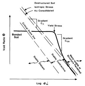
Note that the gradient,  $C_{CS}$ , is a function of  $\mathbf{e}_{O}$  and yield stress, and is not an intrinsic material property, as is  $C_{C}$
