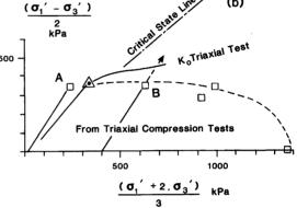
Fig. 6.2. Yield stresses observed in tests on residual soils; (a) residual soil from gneiss (Sandroni, 1981); (b) residual soil from basalt (Vaughan *et al.* 1988).
