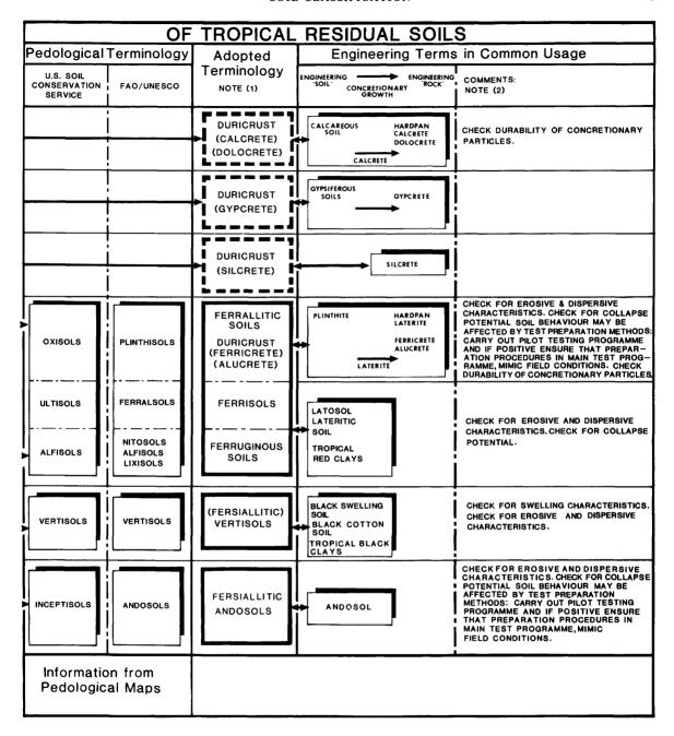
Note (2): The notes in the final column are intended as an early indication of typical behavioural characteristics associated with certain soil groups. Detailed discussion of laboratory testing procedures and engineering behaviour is given in Chapters 5 and 6.
