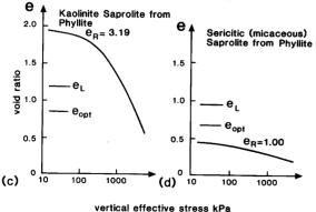
Fig. 5.3. Examples of void ratio used as an index (after Vaughan et al. 1988).
