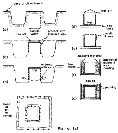
Fig. 5.8. Stages in taking and protecting a block sample.
