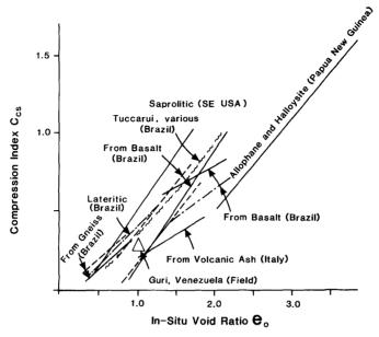
Fig. 6.6. Relationships between compression index,  $C_{CS}$ , and initial void ratio,  $C_0$  (after Wallace 1973; Lacorda et al. 1985).
