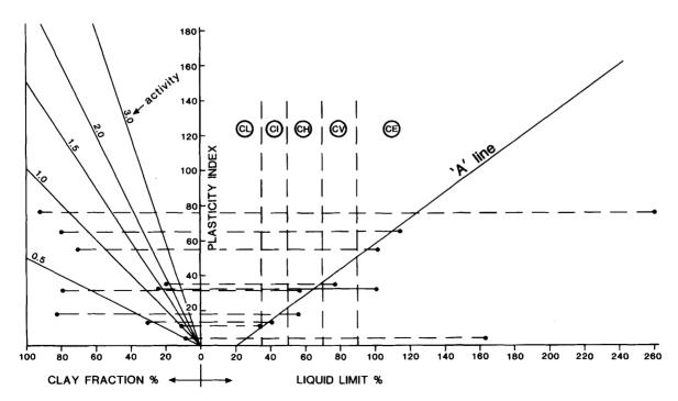
Fig. 5.2. Examples of classification by plasticity and clay fraction.
