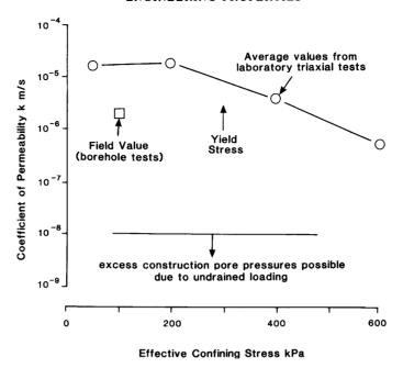
Fig. 6.8. Variation of permeability with confining stress: residual soil from gneiss at Guri Dam (after Medina & Liu 1982).
