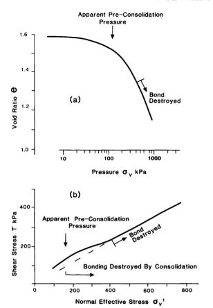
Fig. 6.1. Apparent pre-consolidation pressure (Vargas 1973); (a) observed in the oedometer; (b) influence on drained shear strength in direct shear.
