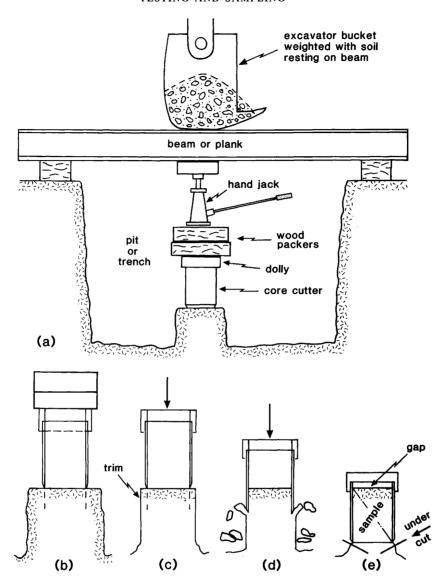
Fig. 5.9. Jacking undisturbed core-cutter sampler.
