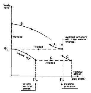
Fig. 5.6. Measurement of swelling characteristics of expansive clays.
