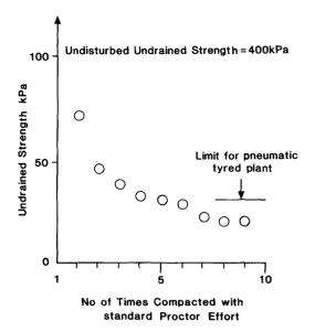
Fig. 6.9. Effect of repeated laboratory compaction on undrained strength of porous residual soil from basalt (Mauritius).
