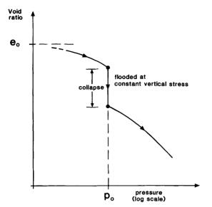
Fig. 5.7. Behaviour of a collapsing soil.
