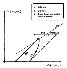
Fig. 5.5. Failure of residual soils with bonding, following different stress paths.
