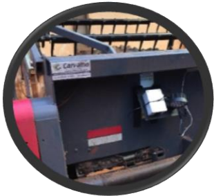
Cameras installed behind harvester platform
