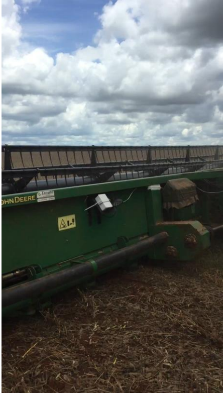
Cameras installed behind harvester platform
