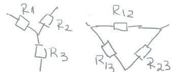
$$R_1 = \frac{R_{12} \cdot R_{13}}{R_{12} + R_{12} + R_{23}} = \frac{R^2}{3R} = \frac{R}{3}$$
