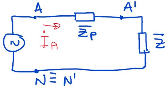
$$\dot{I}_A = \frac{\dot{V}_{AN}}{\bar{Z}_P + \bar{Z}} \quad ; \quad \dot{I}_B = \frac{\dot{V}_{BN}}{\bar{Z}_P + \bar{Z}} \quad ; \quad \dot{I}_C = \frac{\dot{V}_{CN}}{\bar{Z}_P + \bar{Z}}$$
