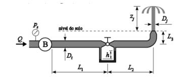
$$\left(\frac{p_a}{\gamma} + \frac{\alpha V_t^2}{2g} + z_a\right) - \left(\frac{p_d}{\gamma} + \frac{\alpha V_t^2}{2g} + z_d\right) = K_{valv} \frac{V_t^2}{2}$$
