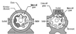
Figura 6 - Bomba de carretos internos http://www.hydraulicspneumatics.com/
