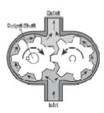
Figura 20 - Motor hidráulico de carretos <a href="http://www.hydraulicspneumatics.com/">http://www.hydraulicspneumatics.com/</a>
