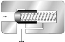
Figura 23 - Válvula de segurança <a href="http://www.hydraulicspneumatics.com/">http://www.hydraulicspneumatics.com/</a>
