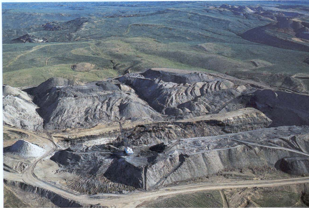
FIGURE 16.9 Open-pit coal mine in Wyoming. The land in the foreground is being mined and the green land in the background has been reclaimed following mining.
