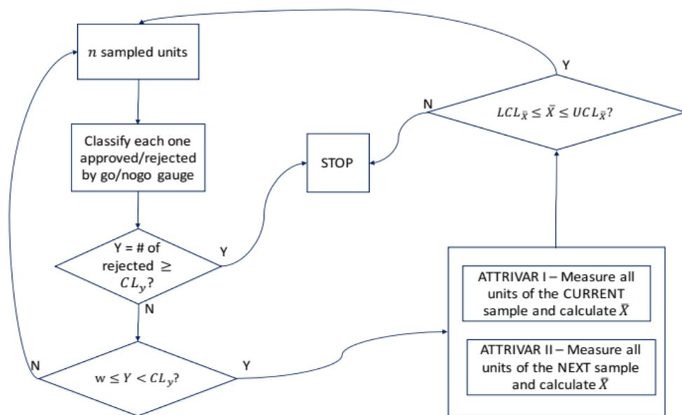
Figure 7: Inspection Procedure
