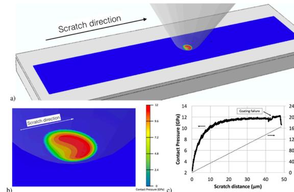
Fig. 14. Contact Pressure at the coating promoted by the indenter movement: a) Instantaneous spatial distribution of the contact pressure; b) detail of the contact region and c) evolution of the contact pressure with the ramping load during the scratch test.
