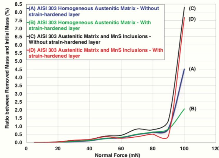
Fig. 6. Numerical results of mass removal by abrasion, obtained considering difference in surface finishing and microstructure.
