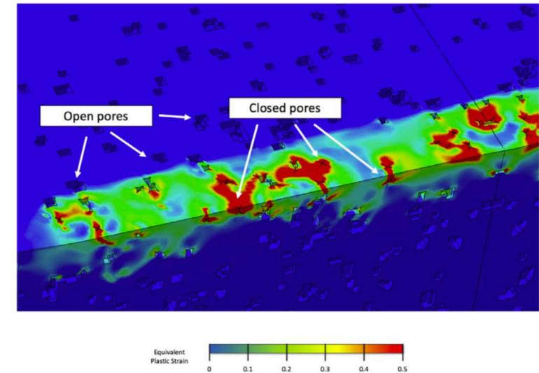
**Fig. 6.** Collapse of the pores by the plastic deformation during the sliding of the sphere. The color field indicates the level of plastic deformation and red regions indicate plastic deformation higher than 50%.
