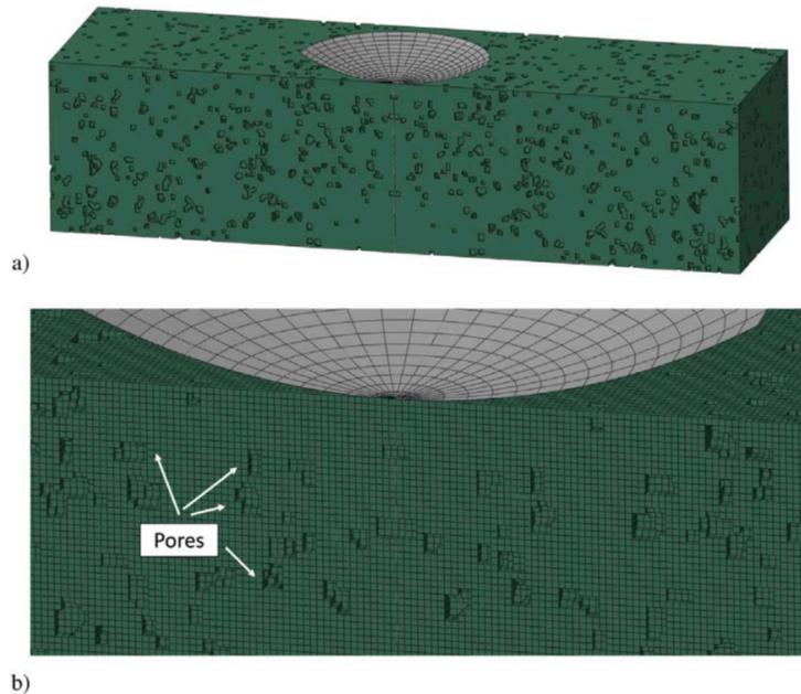
**Fig. 1.** Computational domain for the reciprocating test analyses: a) system composed by an analytical rigid sphere (gray) and a plane counterbody (dark green); b) detail of the system indicating the porosity represented as small voids (regions without elements) in the numerical mesh. (For interpretation of the references to color in this figure legend, the reader is referred to the web version of this article.)
