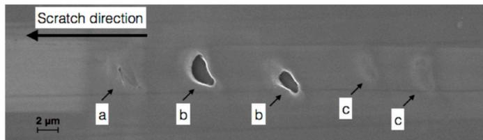
Fig. 8. Microscale scratch track presenting the local typical observed failure modes: a) adhesive and cohesive failures of the coating; b) complete spallation of coating and c) adhesive failure of the coating/substrate interface.
