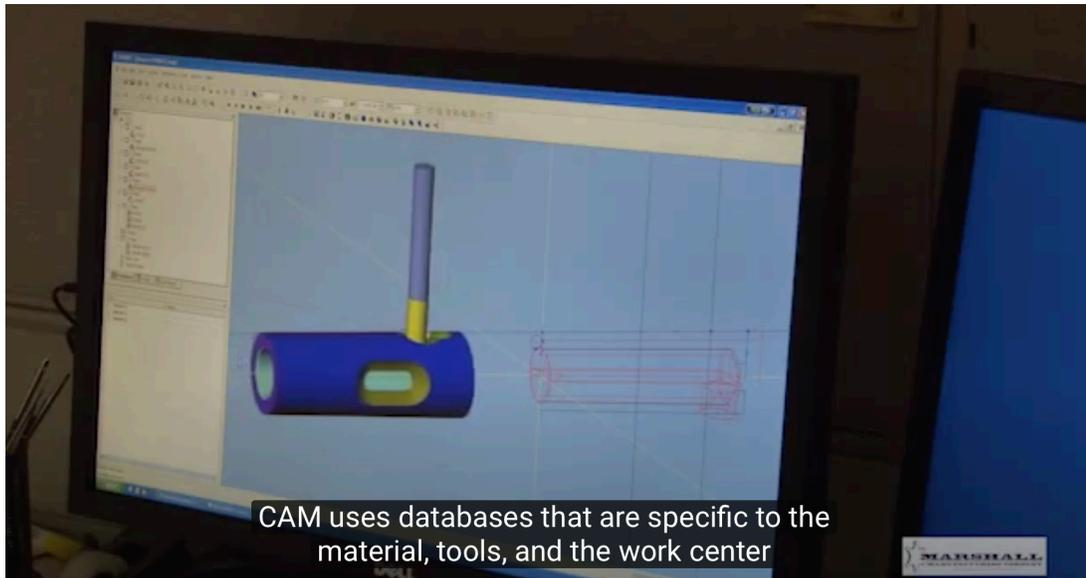
CAM uses databases that are specific to the material, tools, and the work center
