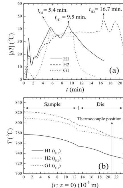
Fig. 3. (a) Estimated temperature difference during the SPS process for the studied samples; (b) the simulated radial temperature profiles for  $z=0$  of samples H1, H2, and G1, respectively (see text for details).
