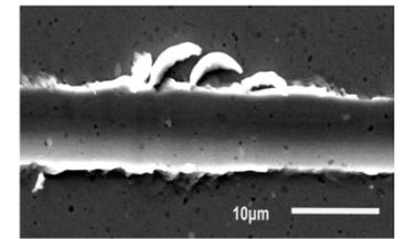
**Chip formation mechanism during cutting:** When the scalar stiffness degradation is unity, the material failure will occur promoting debris such as discontinuous chips agreement with the experimental results.
