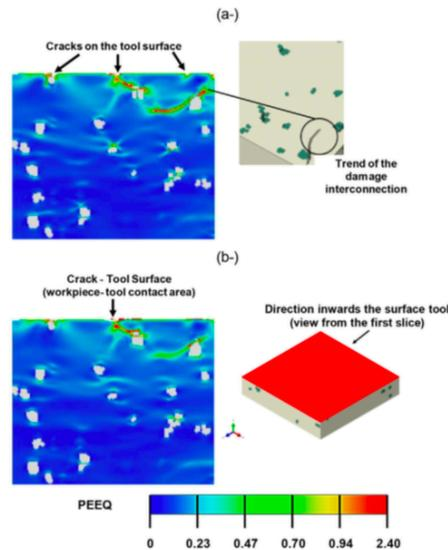
Fig. 11. View from the first slice in the direction inwards the surface tool - Equivalent plastic strain (PEEQ) field after the cooling for the following cases of NbC fracture toughness: 5 MPam<sup>1/2</sup> (a) and 7 MPam<sup>1/2</sup> (b).
