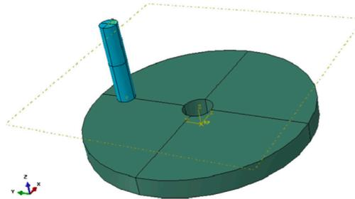
Fig. 1. Geometry of the contact pair pin on disc (tribological system).
