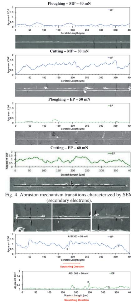
Fig. 4. Abrasion mechanism transitions characterized by SEM (secondary electrons).
