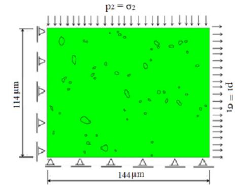
Fig.7. Microstructure boundary conditions and loads applied
